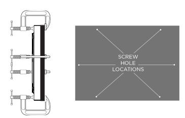
If readjustment is necessary loosen all 6 screws, reposition the panel and re-tighten the screws.
