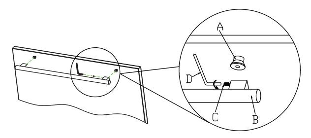
Push the handle tightly against the door and tighten both of the 2 set screws (C) with the hex key (D).
