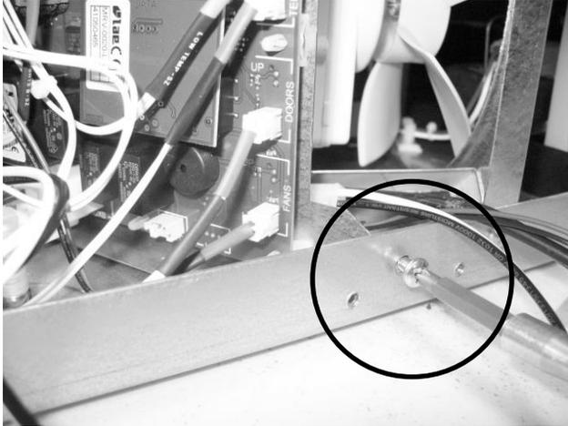
Locate and remove the Phillip's head screw which secures the control board bracket to the cabinet frame.
