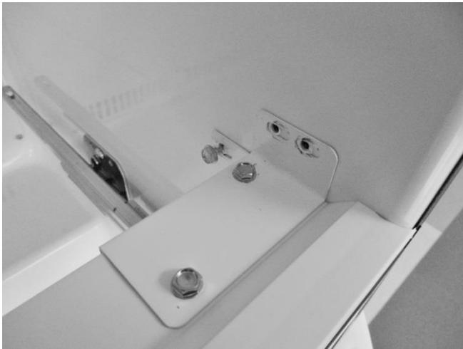
Remove the two top sheet metal screws securing the right hand mullion bracket to the cabinet. Loosen the rear screw. The mullion bracket will stay with the mullion when it is removed.
