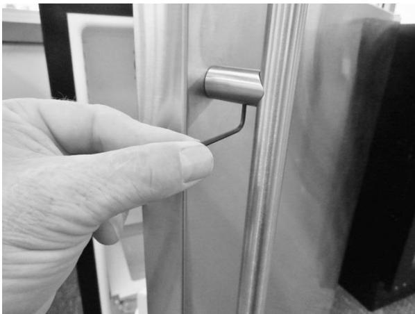
Replace handle stud into the standoff, turn clockwise with the Allen wrench, and snug hex screw finger tight.
