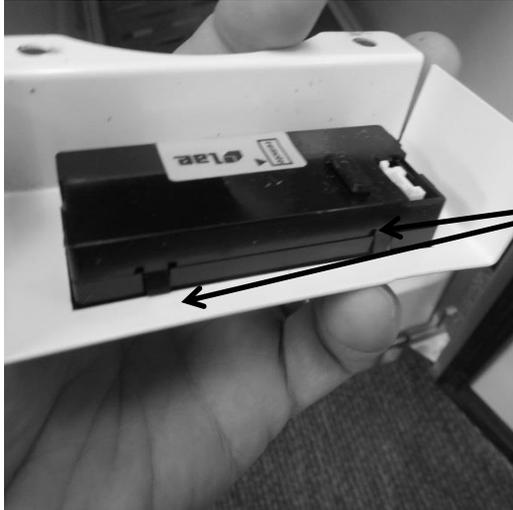
The control can be removed by depressing the four locking tabs (2 on each side) on the control body, with the end of a small screw driver.
