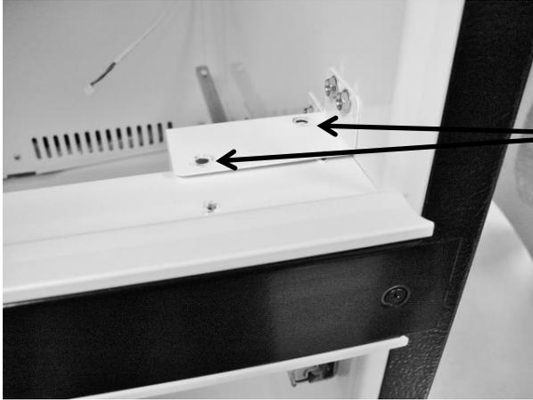
Remove two screws on the **top** of the mullion bracket, and one on the **bottom**.
