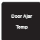
Multiple alarms are possible, i.e.- "Door Ajar" for a prolonged period may trigger a "Temp" alarm, in which case both "Door Ajar" and "Temp" indicators will activate.
