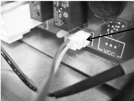
The red and yellow wires at connector 5 (harness B) will plug into the "Aux C" terminal on the main power board.
