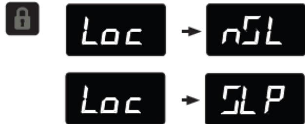
The sleep mode can be disabled if you prefer to have the display on continuously. Press and hold the "Lock" keypad until the display goes past "Loc" and reads "nSL". To enable the sleep mode, repeat the instruction, again going past "Loc" until the display reads "SLP".
