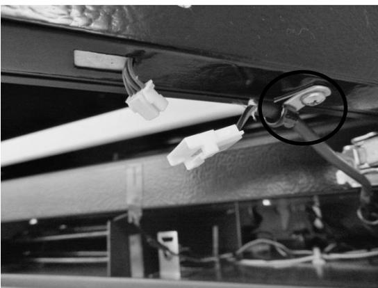
Disconnect communication connector and remove P-clamp and post.
