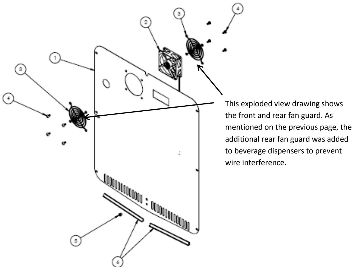
**Air Flow on Beer Dispensers:** The evaporator fan is a draw through design. Specification label will face towards the evaporator when installed correctly. The fan blades will rotate in a counter-clockwise direction as you face the hub.
