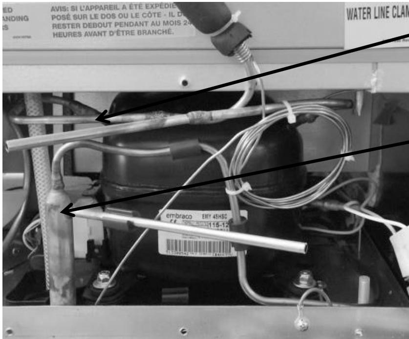
Install and braze the ¼" suction line extension (jumper tube) into the compressor and new suction line.
