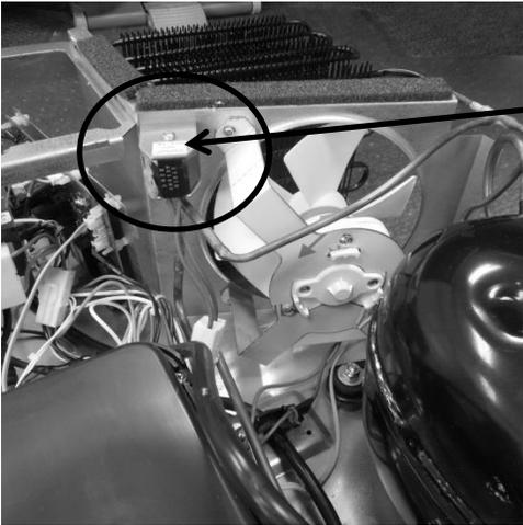
Hot gas valve is located on the rear of the condenser shroud.
