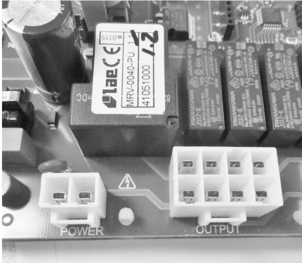
**Connectors J1 and J7: See wiring diagram and schematic included in section 19.8.**
