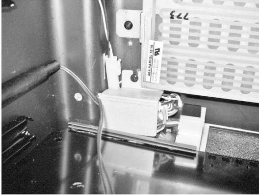
Remove the cover which isolates the electrical connectors.
