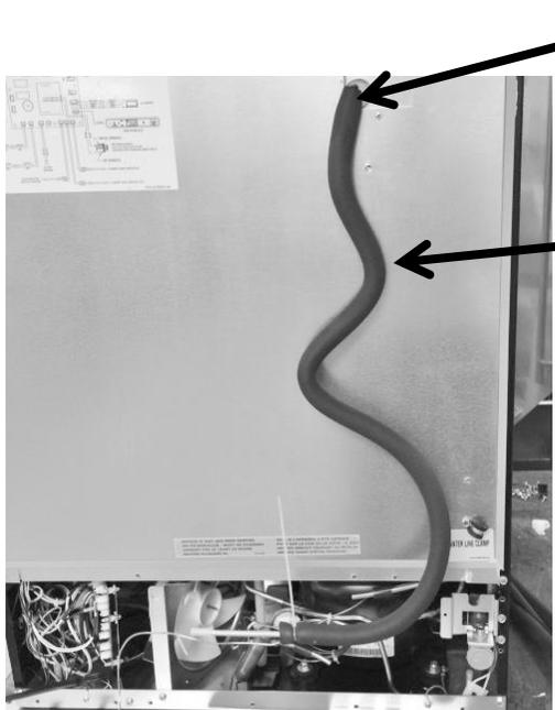
**⚠ CAUTION:** This bend must be made with caution to prevent collapsing, pinching, or restricting the tubing radius.
