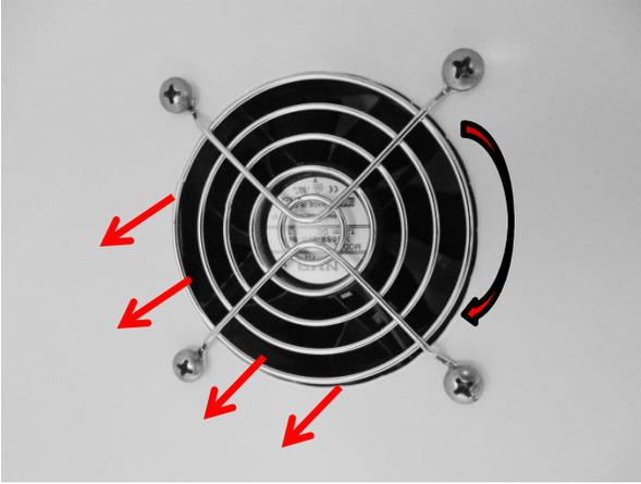
**Most Models:** Evaporator Air Flow: Fan is a blow through type. Specification label facing forward, the blade rotates clockwise as you face the hub.
