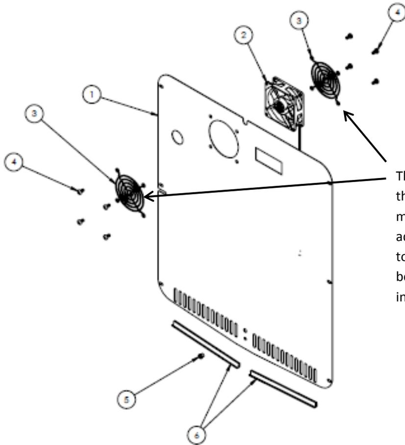
This exploded view drawing shows the front and rear fan guard. As mentioned on the previous page, the additional rear fan guard was added to outdoor beverage centers and beverage dispensers to prevent wire interference.
