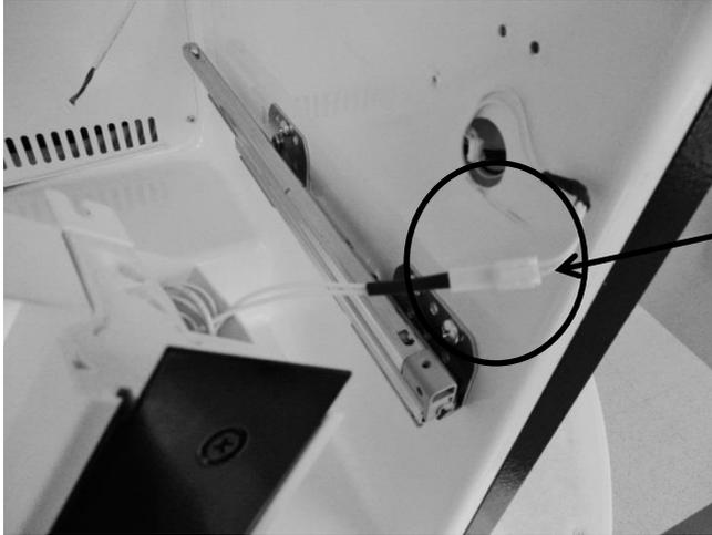
Pull mullion carefully away from cabinet. Disconnect the LED light connector (white wires extended from mullion to the cabinet liner).
