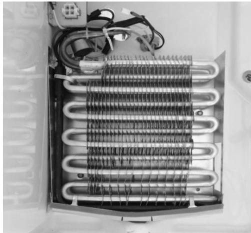
Install the 2 drain pan screws to secure the evaporator assembly. REMEMBER to stuff permagum into the 1" hole drilled for the heat exchanger.
