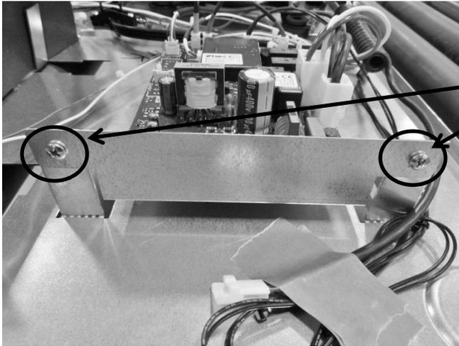
Note the two Phillips screws securing the front of control housing assembly.
