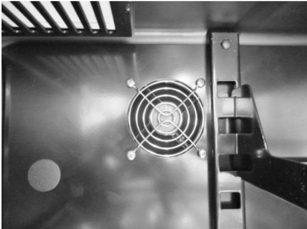
Fan location – do not attempt to remove from this view. Remove coil cover first.
