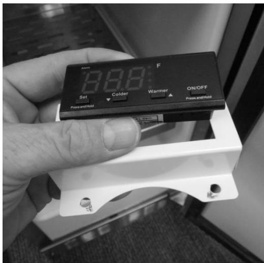
The control can now be removed through the front of the housing.
