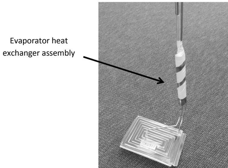
1. Straighten out the tubing on the new assembly so that it can be installed.
