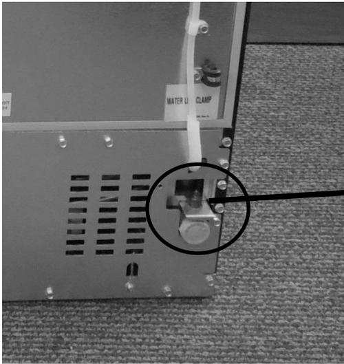
Supply water inlet: ¼" compression nut with coupling.
