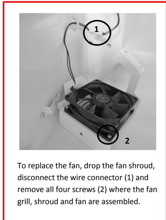
To replace the fan, drop the fan shroud, disconnect the wire connector (1) and remove all four screws (2) where the fan grill, shroud and fan are assembled.
