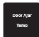
Multiple alarms are possible, i.e.- "Door Ajar" for a prolonged period may trigger a "Temp" alarm, in which case both "Door Ajar" and "Temp" indicators will activate.
