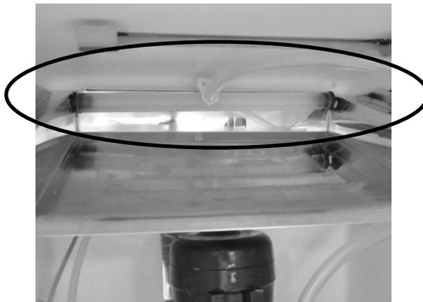
The distribution tube is located above the evaporator plate and is held in place with the two black rubber plugs that are inserted into each end and placed into the holes on each end of the evaporator plate.
