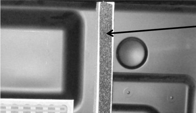
**VIEW:** Styrofoam air channel insert.
