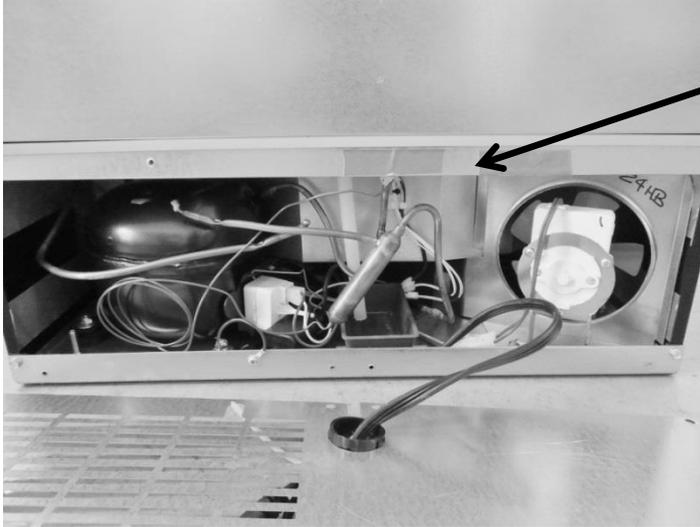
View of the machine compartment components with back panel removed. NOTE the location of the compressor, drain, condenser fan, and filter drier.
