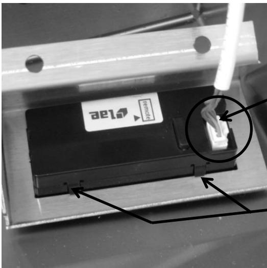
To disconnect, press the release tab on the side of the wire connector and remove the communication cable.
