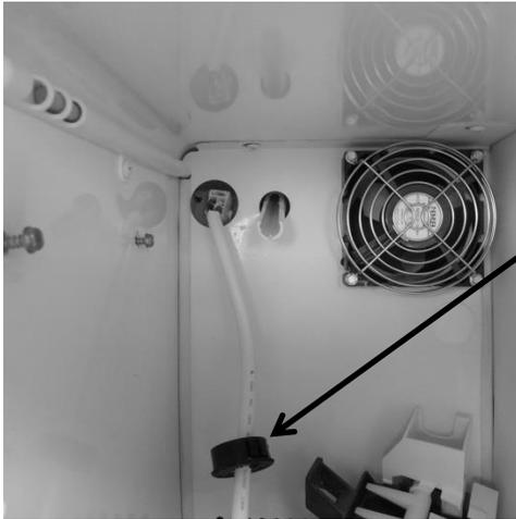
Remove the black wire grommet on the rear of the freezer cover. This will expose the connector for the ice maker harness.
