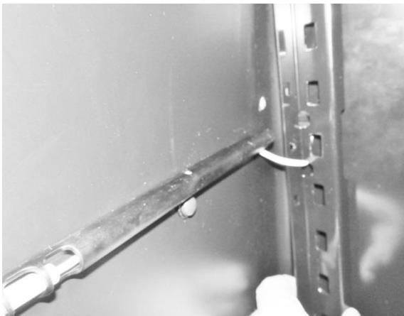
Beverage center only: The cabinet thermistor will have to be removed from its shield to allow it to pass through the removed cantilever bracket.
