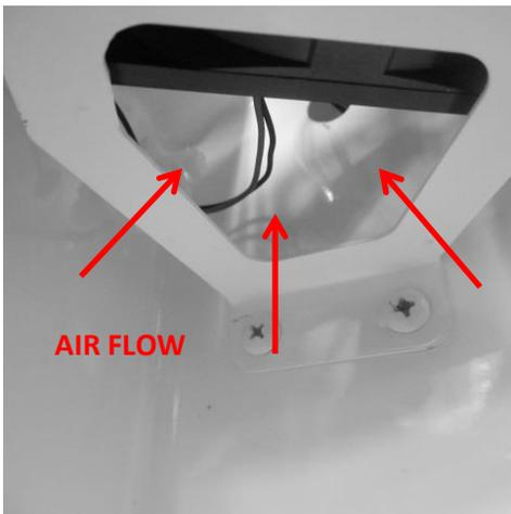
The bottom of the fan assembly is open to recirculated air from the compartment. The air is then pushed out into the compartment through the fan blade.
