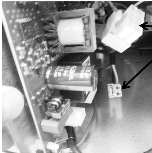
Tip board at a 90° angle and disconnect the two large white connectors from the power board.
