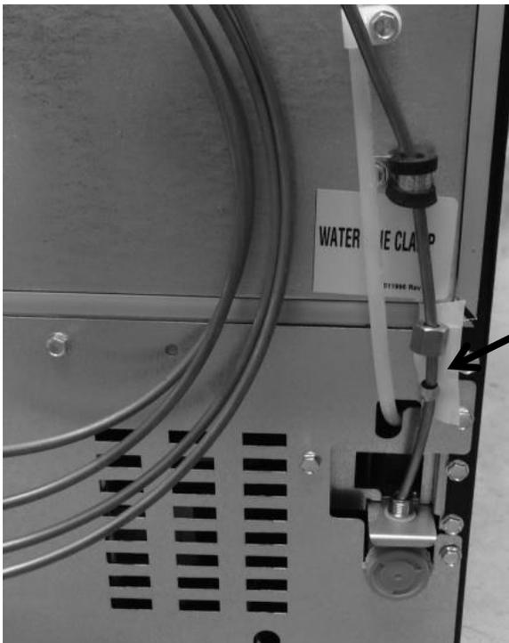
Install water supply line to the water valve, seat coupling and tighten the compression nut to the water valve.
