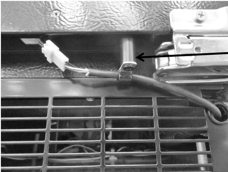
**The cable post is used only on articulating hinge doors.** Its purpose is to keep the communication cable from being pinched by the hinge. The p-clamp, post and harness connector must be detached from the door to accommodate door removal.
