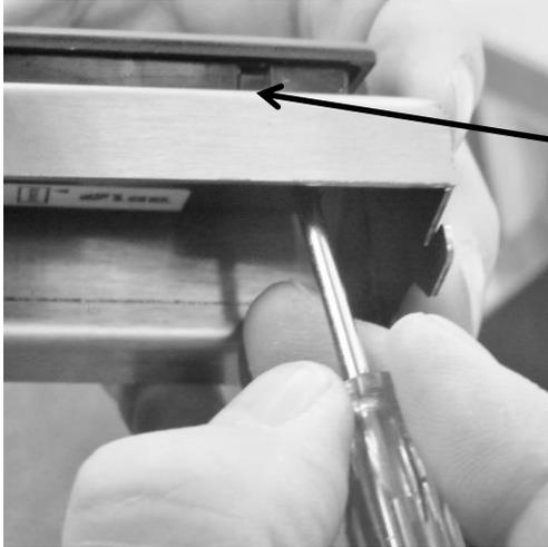
The control can be removed by depressing the four locking tabs (2 on each side) of the control body, with the end of a small screw driver. This will allow the control to be removed from the front of the housing.
