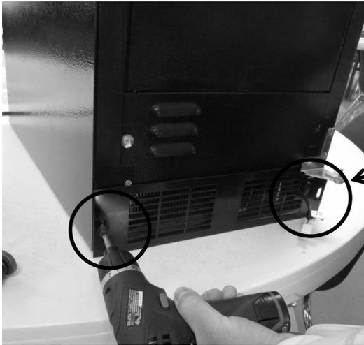
Remove each Phillip screw on both ends of the toe grill.
