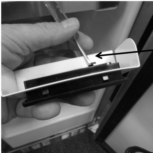
A small screw driver is used to release the locking tabs on the control from the control housing.
