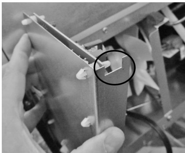
Recess on the bottom of the mounting bracket.
