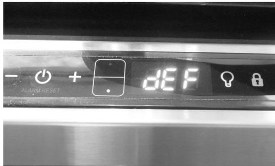
Defrost can be achieved either automatically or manually. A manual defrost can be activated by holding the minus and lock keys simultaneously for a period of three seconds. Once defrost is activated the Use Interface will flash "dEF" three times before showing an uninterrupted "dEF". More information is available in Section 5.
