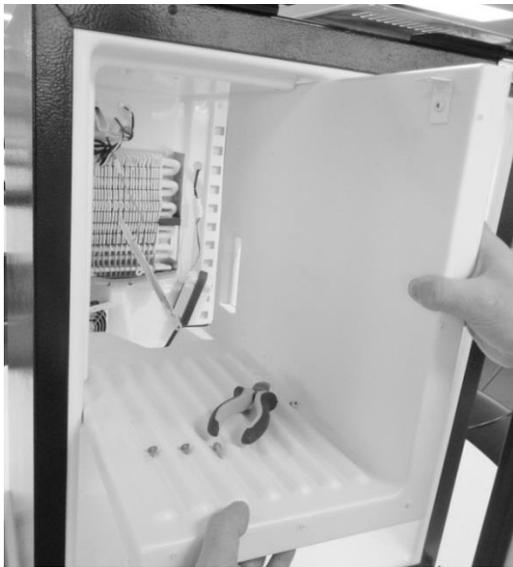
The freezer partition can easily be removed for access to the evaporator section. Remove the three screws from the taps (2 on the top vertical and 1 on the left horizontal corner) where they are screwed into the cabinet.
