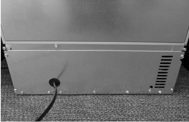
Remove all perimeter 5/16" screws that secure the back panel – DO NOT remove the 5/16" hex screws in the bottom left and right hand side corners, or the Phillips head ground screws.
