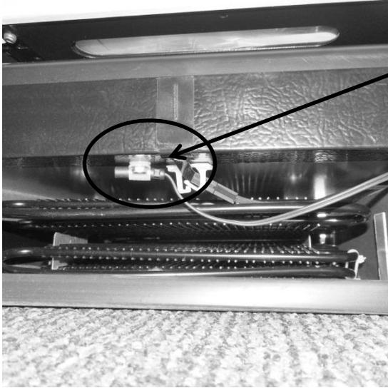
Location of ***ambient thermistor*** is located behind the toe grill and secured to the top of the machine compartment, centrally located in the condenser intake air.
