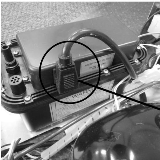
The black power plug on the pump connects to the main power board.
