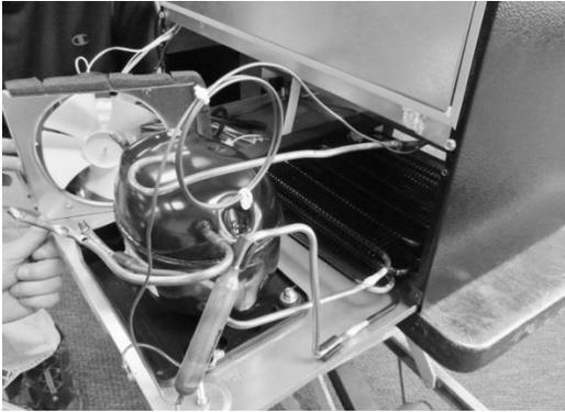
Slide out the bottom of the machine compartment far enough to unsolder condenser lines.
