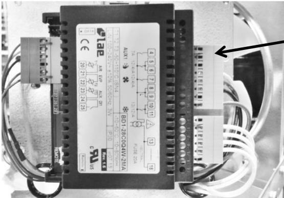
Visual of the main control board attached to its mounting bracket with all wire harnesses connected.
