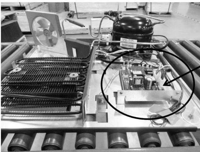
**FOR REFERENCE:** The bottom base assembly is shown to help identify component locations. The control housing assembly is circled in red.
