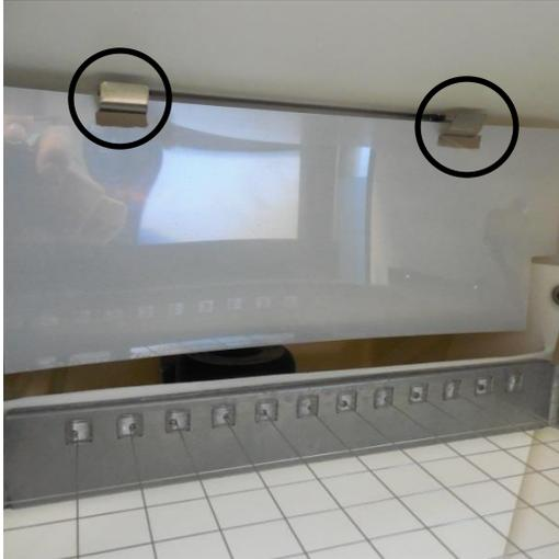
The water shield is slotted and suspended by the two hooks mounted at the rear top of the ice machine.
