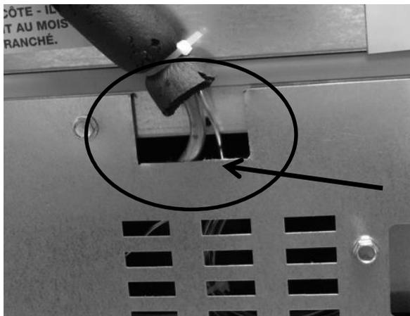
Notch out a clearance hole on the rear access panel to accommodate the suction line and capillary tube.
