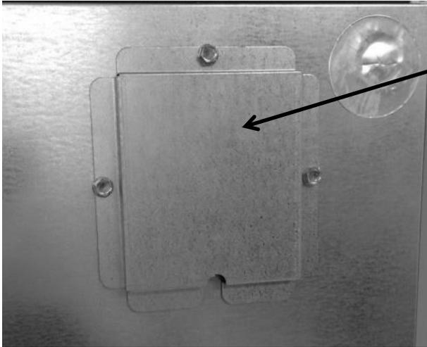
Remove access cover in top rear, right hand corner. Remove insulation under cover and keep for use later.
