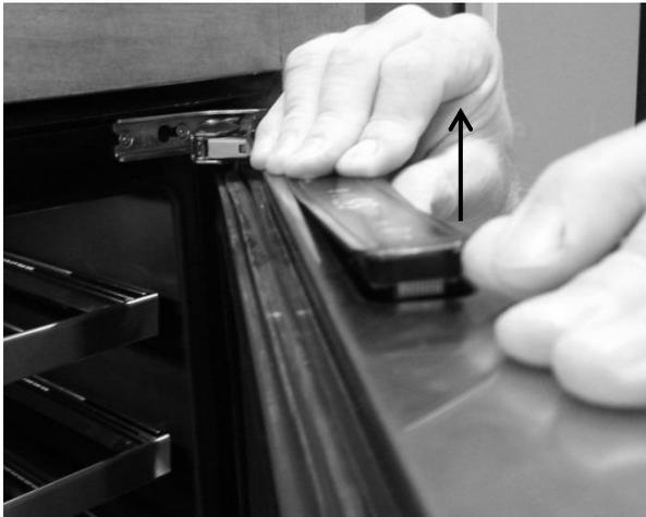
Lift up on the left hand side of the user interface display. Once the display is unseated, raise it high enough from the door boot to disconnect the wire harness.
