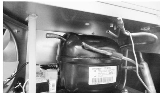
**Size and cut the suction tube extension to connect the compressor to the suction line.**
