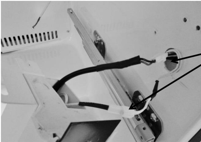
Connect both the light and heater wires from the mullion assembly to the wires leading from the cabinet.
