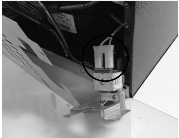
Attach water valve to rear cabinet flange. Replace cover to machine compartment.
