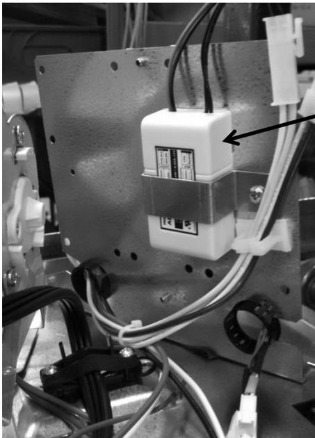
**12 VDC Power Supply** – Serves the *evaporator fan*. The power supply is located on the rear side of the main power board bracket.
