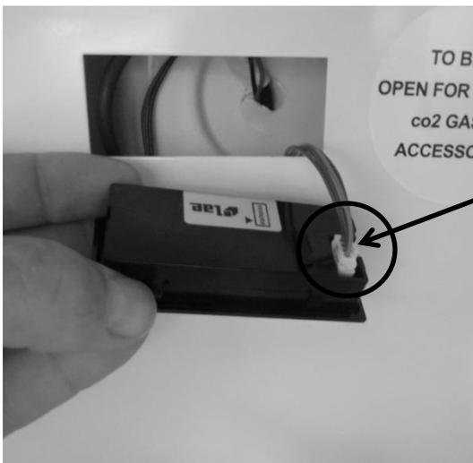
Disconnect the wire harness from the control by pressing the release tab on the outside of the connector.
