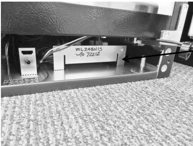
Control housing assembly: The main power board is located in the front, right hand side, behind grill (beer dispensers only).
