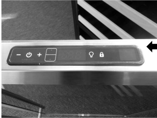
**User Interface Display:** Features dual compartment temperature set point option on display.
