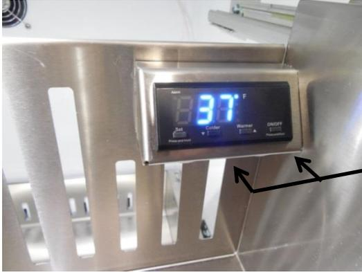
On Refrigerated Drawers: Follow the steps below. Two mounting screws are located on the bottom flange of the control housing.
