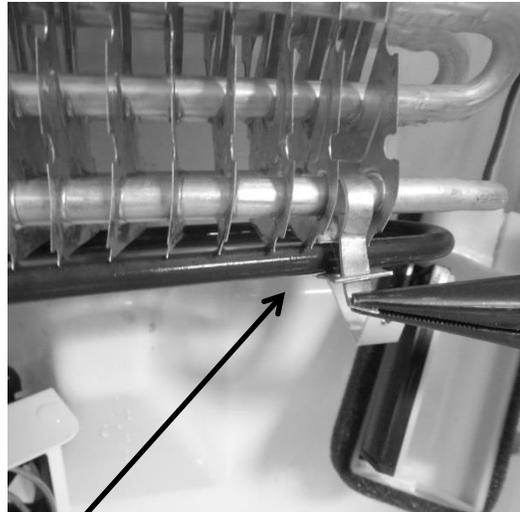
Remove the tin tie wraps that secure the heater next to the evaporator.
