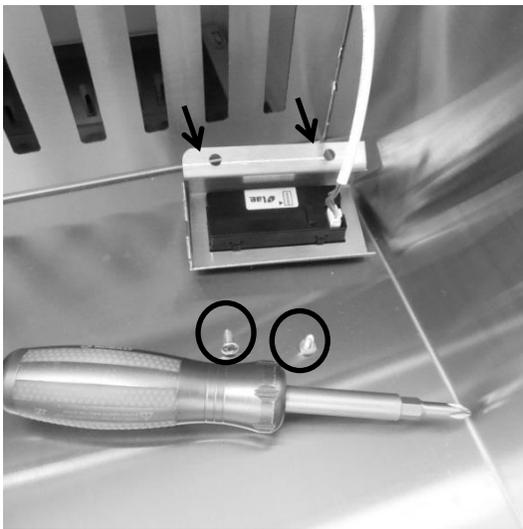
To access the control, remove the two screws on the bottom housing flange. Grasp the control and pull away from the drawer.
