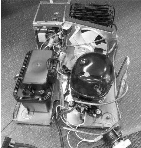
The drain pump sits at the rear, left hand side of the machine compartment base assembly.
