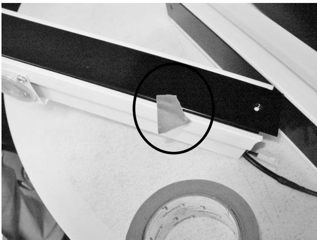
Prior to installing the new mullion assembly, center the black painted strip over the plastic mullion. Use a piece of tape on each end to temporarily hold the assembly together.
