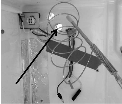
Feed the capillary tube and suction line of the new evaporator assembly (inside to the outside) through the 1" hole.
