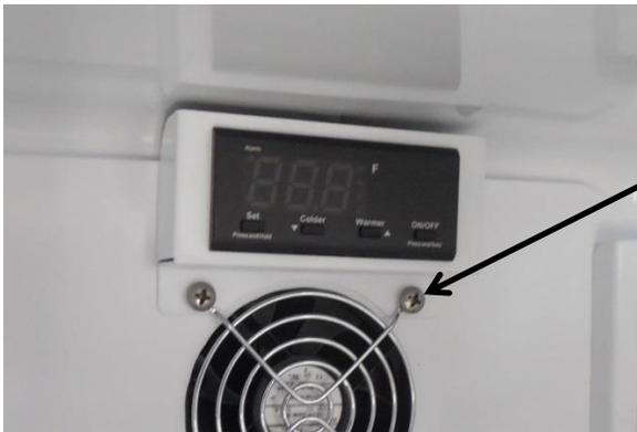
To access the control, remove the two screws on the bottom housing flange. These screws also secure the fan grill and motor to the evaporator cover.
