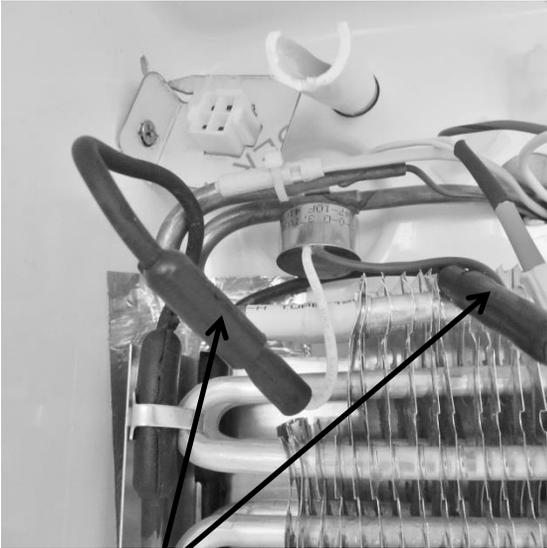
Locate defrost heater connections.
