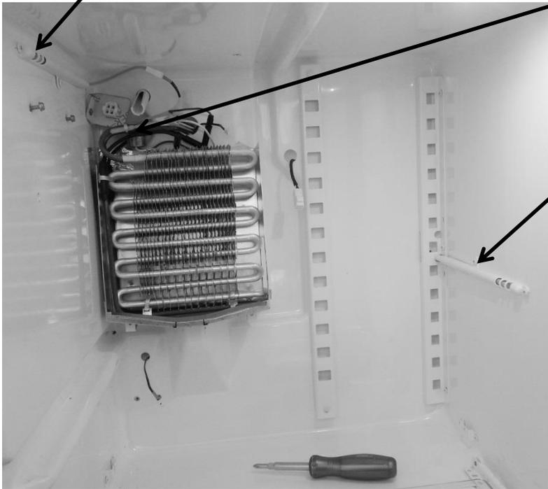
The defrost thermistor is mounted on the evaporator outlet. The evaporator is located behind the freezer compartment.
