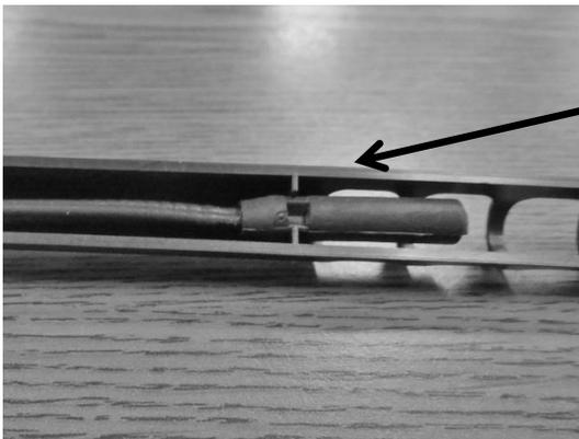
**Bin Thermistor:** NOTE the locator slot inside the thermistor shield. The grooved thermistor bulb fits firmly in place inside the shield.
