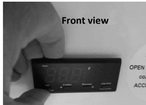
To remove the control: Insert your fingers on the top of the control and press downward. This will release the two bottom tabs. Pull the top of the control outward from the evaporator cover.
