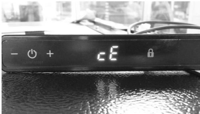
The photos to the left show a definite communication error (cE), the result of this was a broken brown wire in the cable itself. This can occur inside a connector at the user interface, the bottom of the door, the main control board, or a broken wire anywhere in the cable itself.
