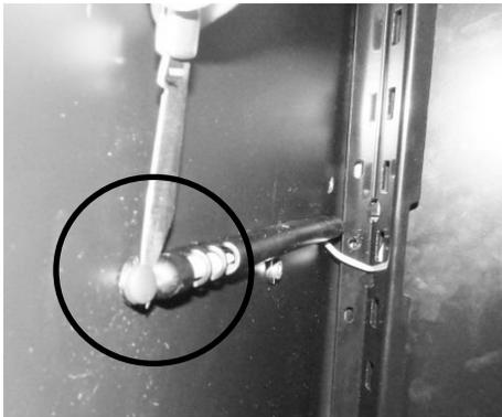
← A knife or small putty knife is used to pop each snap cap off the screw heads. Place the blade on the rear base of the cap and lightly pry upwards.
