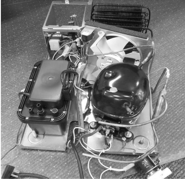
Mechanical assembly completely unsoldered and removed from under the cabinet.
