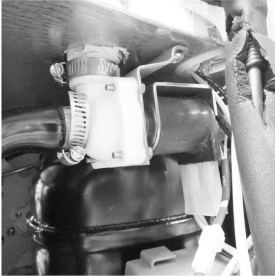
To remove the drain valve, disconnect:
