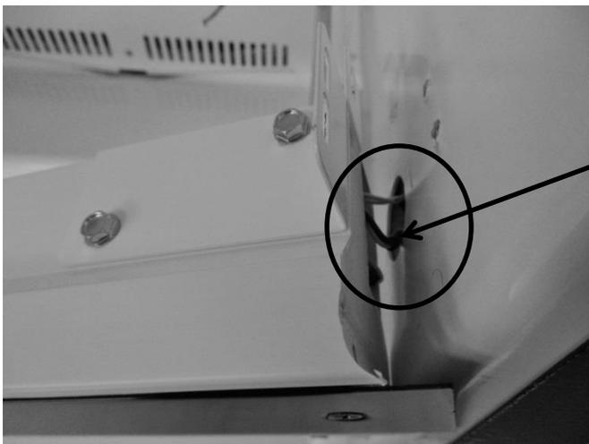
Feed the remaining light and heater harnesses into the mullion assembly.
