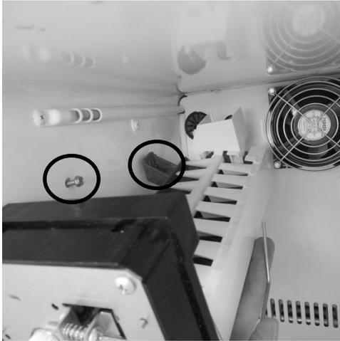
To remove the crescent ice maker, the screws located inside the two upper mounting brackets need to be loosened. There is no need to remove these screws. A third screw on the bottom front of the ice maker body needs to be completely removed.
