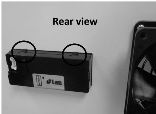
Tab release: Two tabs are located on the top and two on the bottom on the control.
