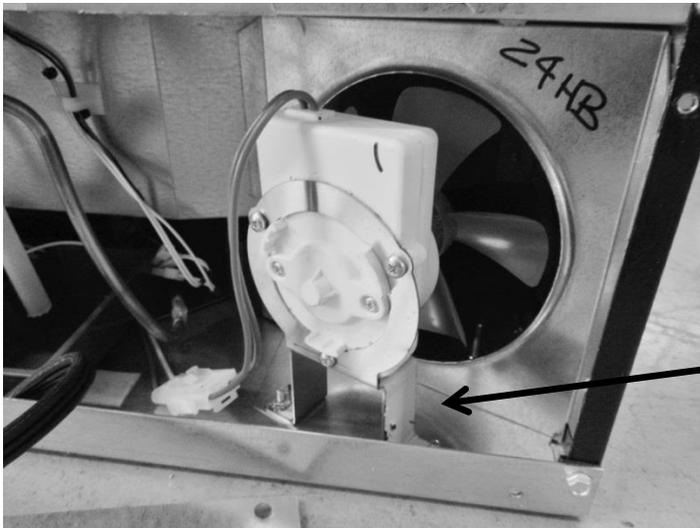
The condenser motor can be replaced by releasing the disconnect plug and removing the nuts holding the mounting bracket to the base assembly.
