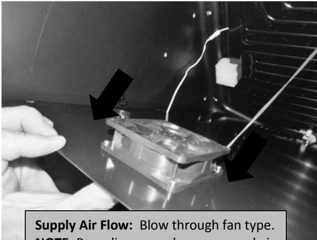
**Supply Air Flow:** Blow through fan type.
