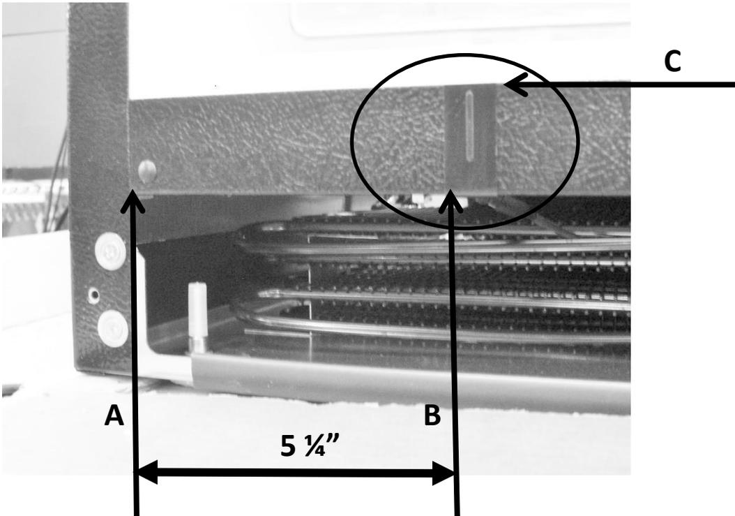
**ALWAYS LOCATE AND POSITION THE SENSOR FROM THE HANDLE SIDE OF THE CABINET.**
