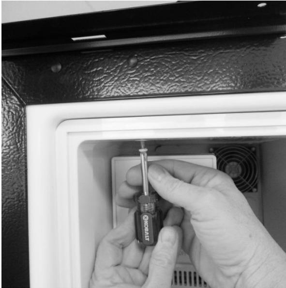
To access to the freezer / evaporator compartment, first remove the freezer door and frame assembly. This will total 6 screws, 5 on the inside perimeter of the door frame, another on the inside upper left hand corner.
