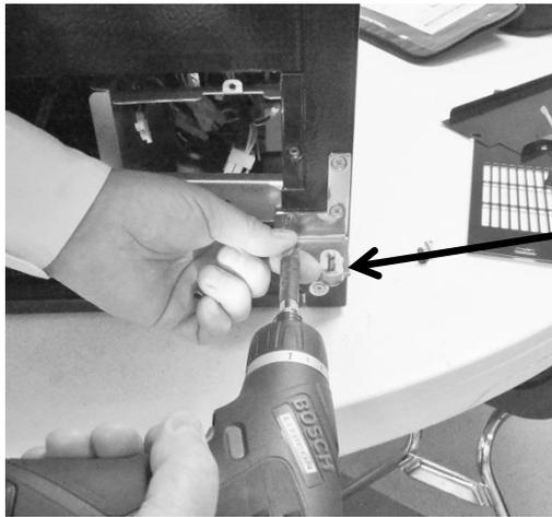
Remove bottom left hand screw from lower hinge.
