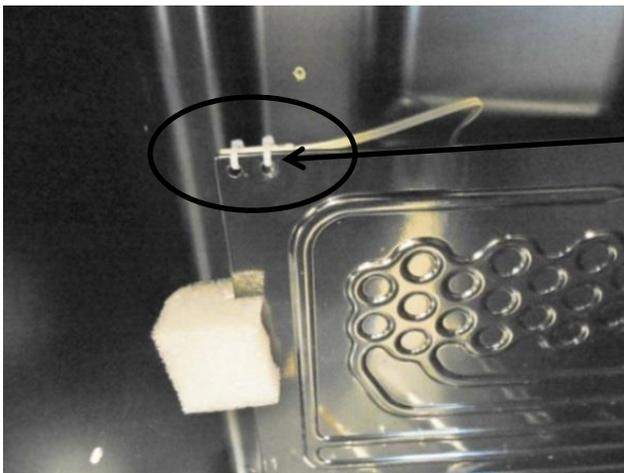
Location of the defrost thermistor: Top left hand corner of evaporator plate.
