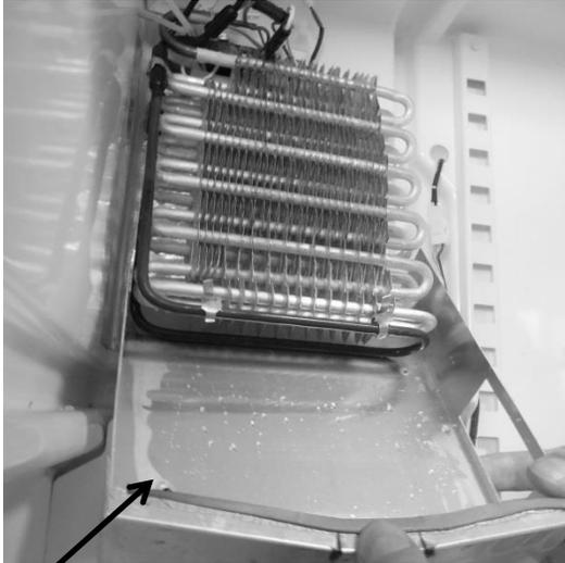
Slide the drip pan down away from the evaporator.
