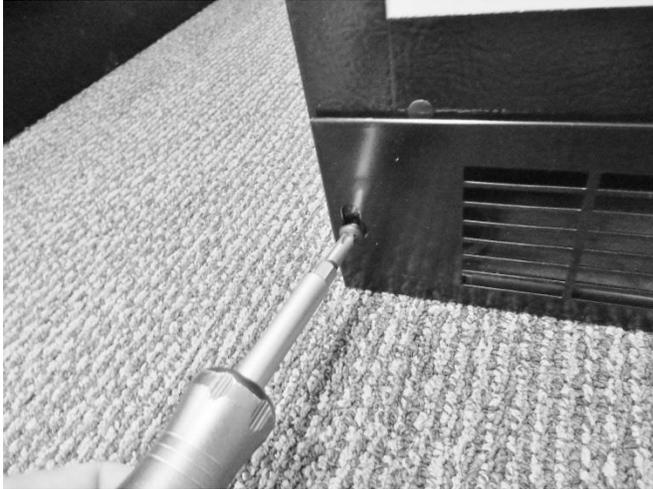
To access the main power board; remove the toe grill.
