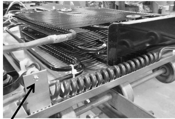
The above bracket is used on LEFT HAND SWING doors to anchor the back end of the communication cable.
