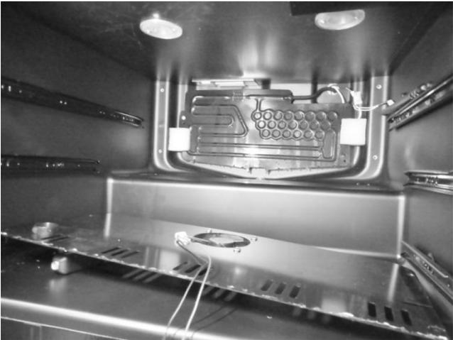
**VIEW:** Lower compartment with rear panel removed. *Center divider is in place.*
