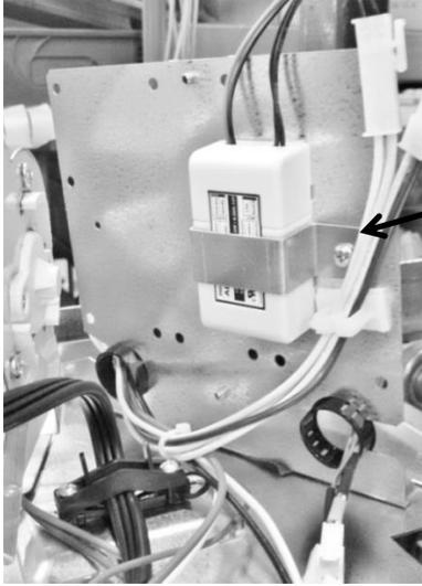
**12 VDC Power Supply** – *Serves the evaporator fan.* Located on rear side of the main power board bracket.
