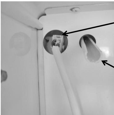
Grasp and squeeze the connector by the release until it disengages. Pull to disconnect.
