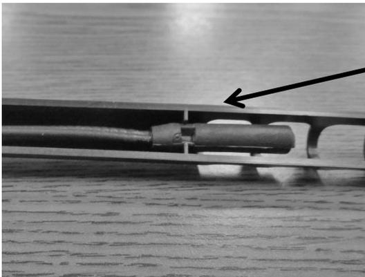
**Cabinet Thermistor:** Note the locator slot inside the thermistor shield. The grooved thermistor bulb fits firmly in the seat created inside the shield.
