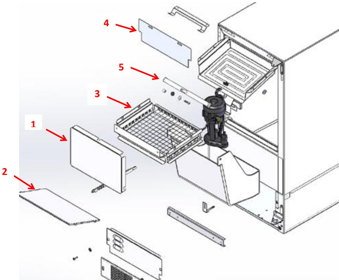
To access the evaporator plate, first remove the following:
