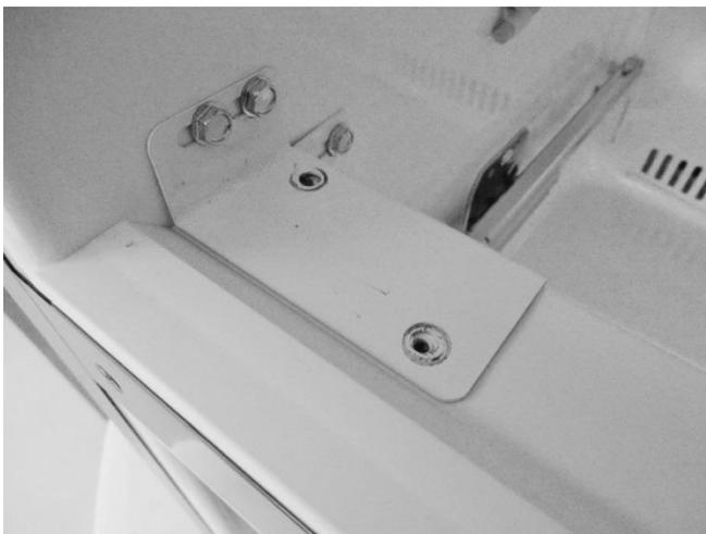
Remove the sheet metal screws on the top and bottom of the left hand mullion bracket. The mullion bracket will stay attached to the cabinet.
