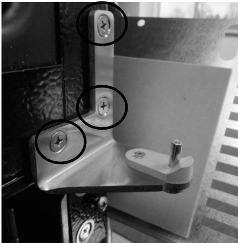
Remove screws to replace the door closer assembly.
