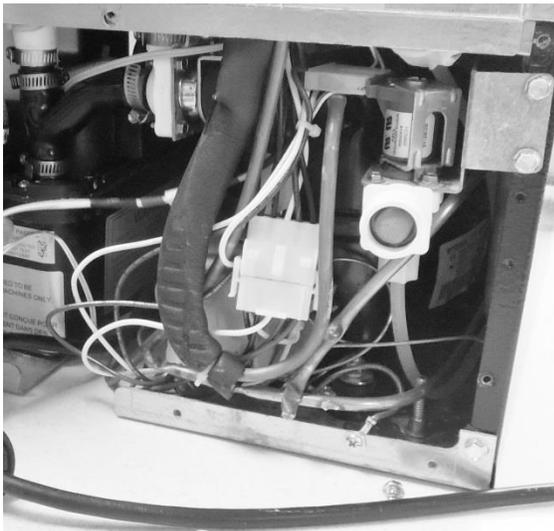
To remove the water valve, disconnect:
