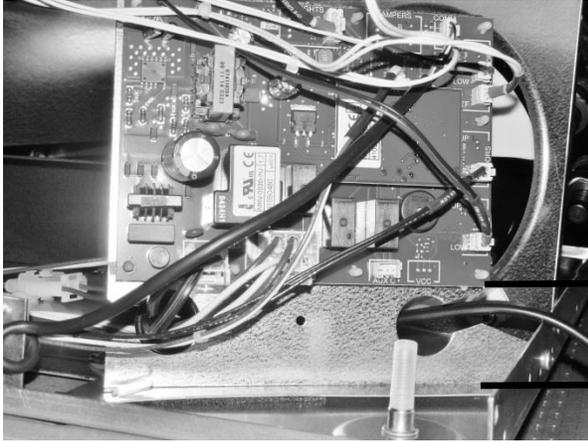
The photo to the left shows the new modified board bracket to extend the mounting height farther away from the cabinet base.
