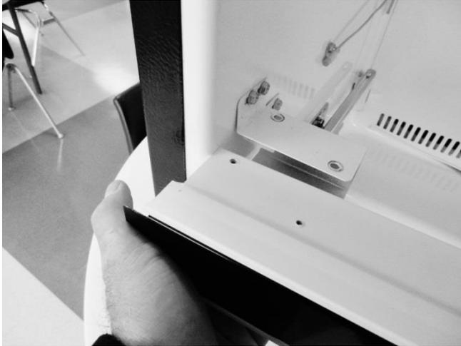
Carefully align both ends of the assembly with the cabinet bracket locations. This will fit firm. Take care not to pinch the LED and heater wire harness, press both ends of the assembly into place.
