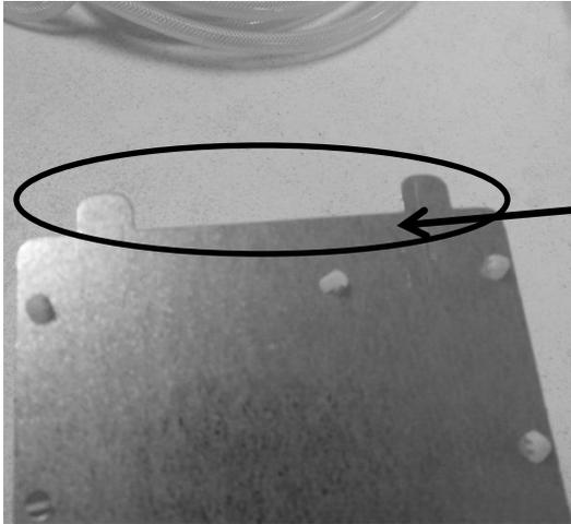
These two photos show both the mounting tabs on the bottom of the main control board bracket and the positioning slots on the adjoining mounting bracket inside the machine compartment.
