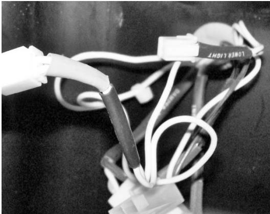
***NOTE: Each wire with a connector is labeled with a piece of shrink wrap tubing in regards to its termination point.***
