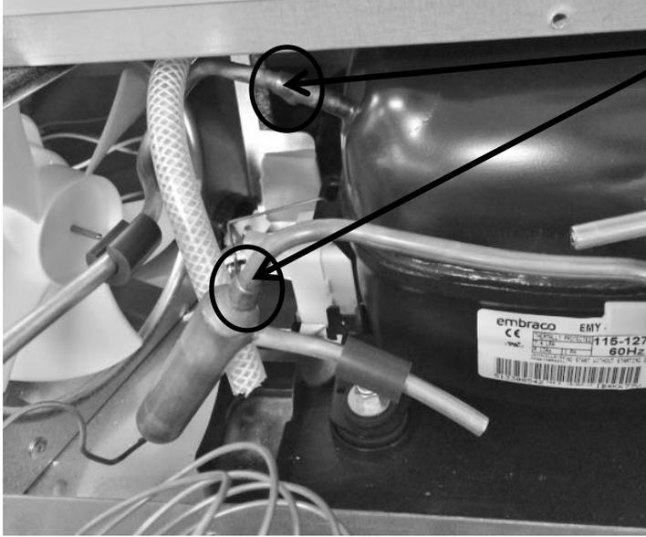
Un-braze the remaining suction line and the filter drier at these joints.
