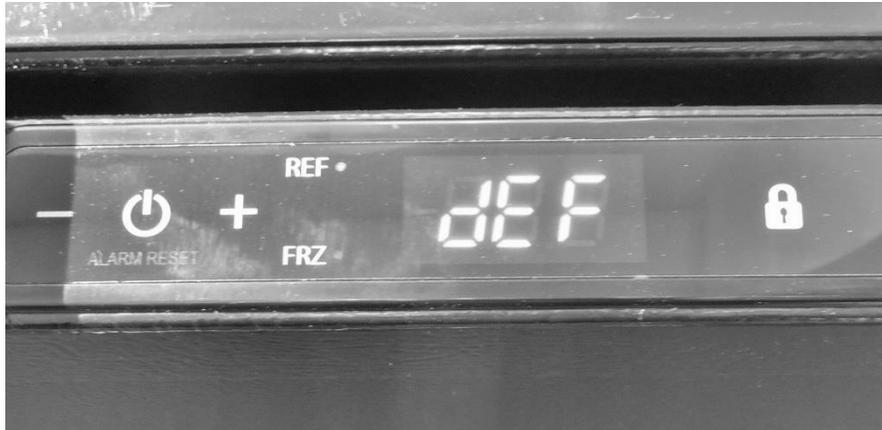
Defrost can be achieved either automatically or manually. A manual defrost can be activated by holding the minus and lock keys simultaneously for a period of three seconds. Once defrost is activated the Use Interface will flash “dEF” three times before showing an uninterrupted “dEF”. More information is available in Section 5.
