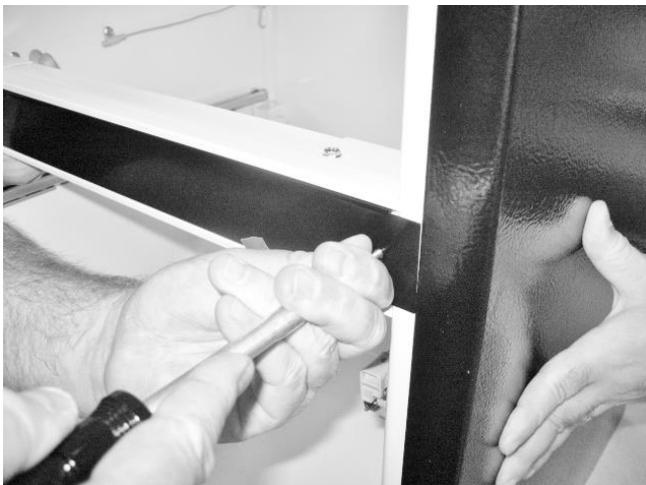
Secure the mullion assembly using the black head screws. Use one screw on each end of mullion, the screw will self-tap into the assembly.
