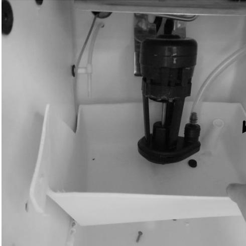
The reservoir can now be removed by lifting off the bottom drain extension.
