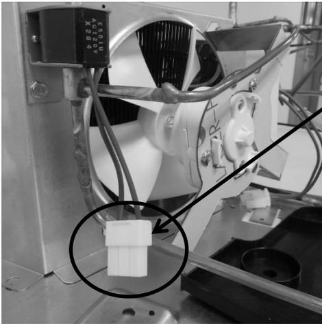
Hot gas valve disconnect is shown in photo.
