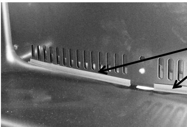
Drip edge on bottom of evaporator cover.
