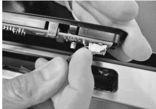
Release locking tab on display connector.
