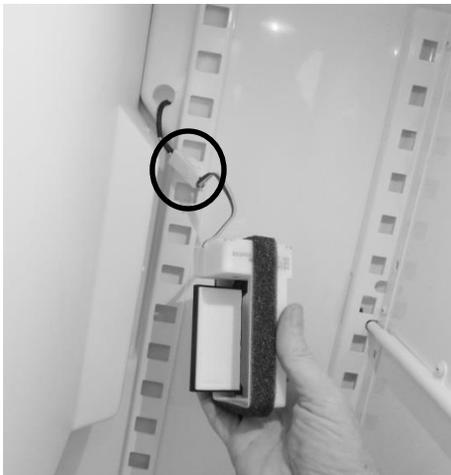
The damper can be grasped and pulled out of the opening. Disconnect the wire connector to replace.
