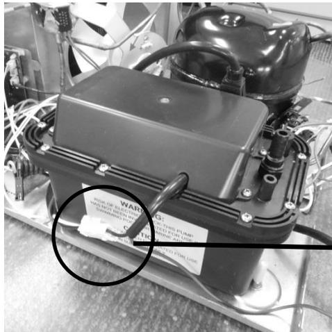
The white connector at the drain pump connects the appliance to the supply voltage receptacle.
