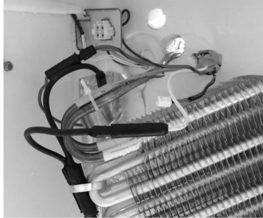
Replace heater, defrost termination thermostat, and zip tie the thermistor to the evaporator.
