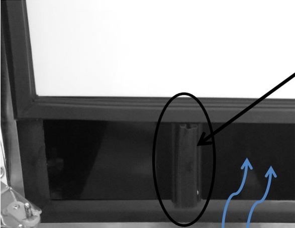
Air recirculation barrier mounted vertically on the bottom of the inside door panel. This allows additional intake air flow into the condenser.
