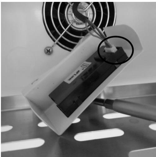
After removing the screws, grasp the control and pull away from the evaporator cover.
