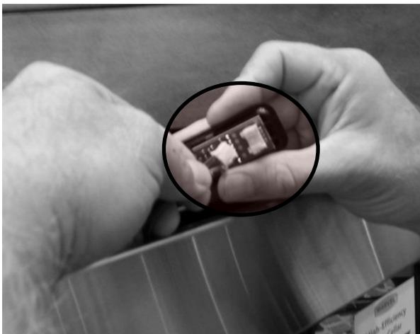
Turn the user interface over, press the disconnect lock and separate the display from the wire harness.
