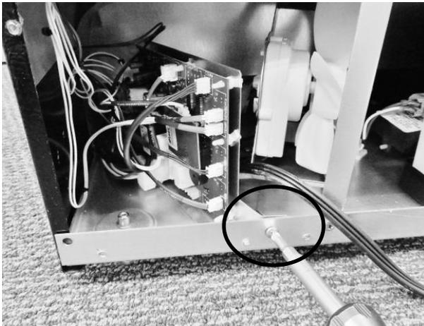
Remove screw holding the control board bracket in place.
