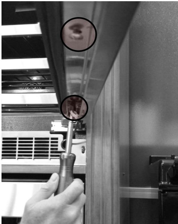
Remove the two Phillips screws on the bottom inside of the door frame.
