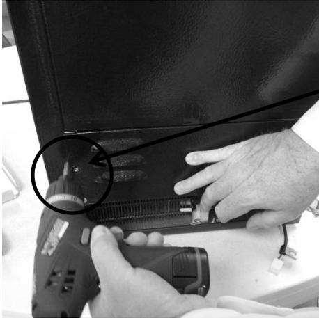
Remove each Phillip screw on each side of the louvered access panel to gain additional access.
