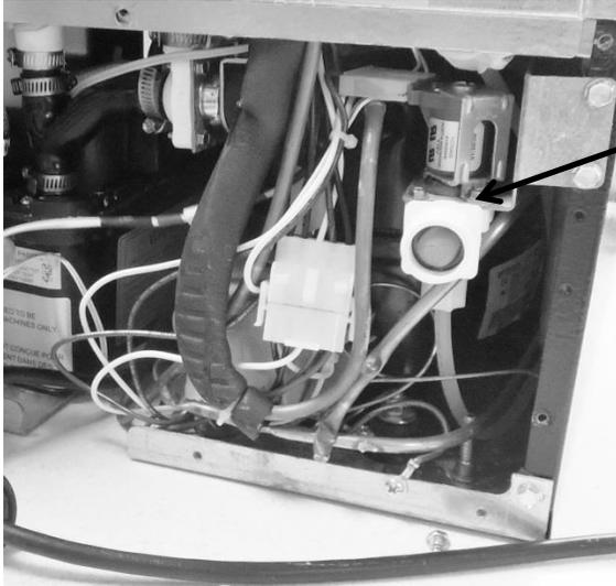
High side thermistor location: The thermistor is located on top of the filter drier inlet (located behind the fill valve). The water valve will have to be removed for access.
