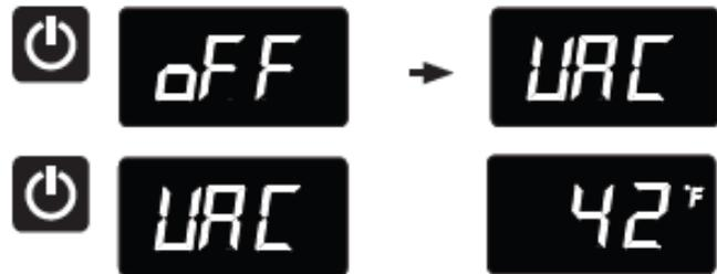
To enter Vacation Mode (with the control out of sleep mode), press and hold the "On/Off" keypad until the display goes past "OFF" and reads "VAC". The display will flash "VAC" 3-times to acknowledge your request, then will display "VAC" continuously until Vacation mode is exited. A power outage will not exit Vacation mode, exiting can only be accomplished manually. To exit Vacation mode and return to normal operation, press and hold the "On/Off" keypad until the control displays the temperature.
