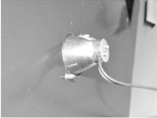
This is a photo of the bottom compartment LED. It was taken after the divider was disassembled. It references the need to carefully finger tighten the bulb when replacing. No clips or backers are used for assembly.
