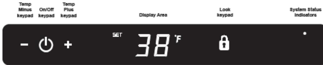
Figure 13 Electronic single zone control
