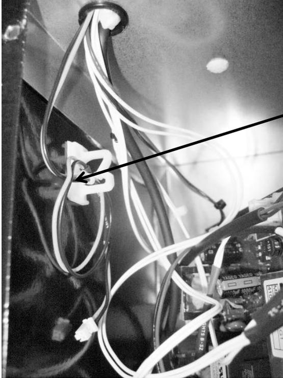
Note the location of the black and yellow mullion heater harness in the machine compartment.
