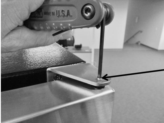
**1/8" hex head.** Turn the screw counterclockwise to remove.
