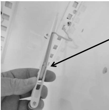
The thermistor bulb is located with the notch on the lower bulb which will nest inside the locating clip on the inside of the thermistor shield.
