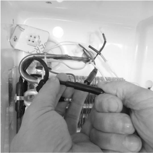
To replace defrost heater, unplug the connections.
