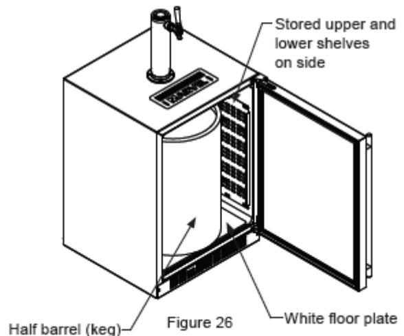
This beer dispensing unit will support one half (½) barrel or one quarter (¼) barrel. The double draft tower units can support two sixth (⅙) barrels of beer. See chart below for quantity of beer in each barrel size.
