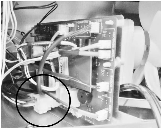
Disconnect the power connector at the bottom, left rear of the control board. See below photo for reference.
