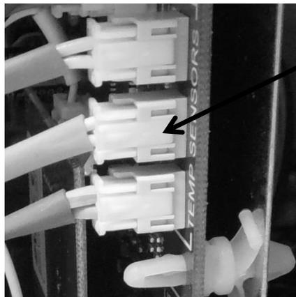
Example: Clip release on side of terminal disconnects. Press to release. A click will be heard when disengaged from control board.
