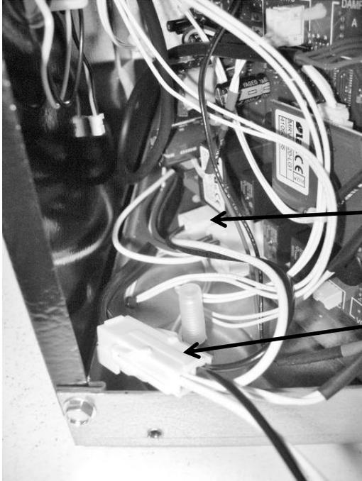
View of wiring harness A with connectors "1" and "2"
