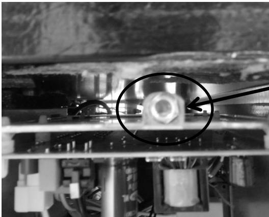
Remove screw holding the control board bracket in place.
