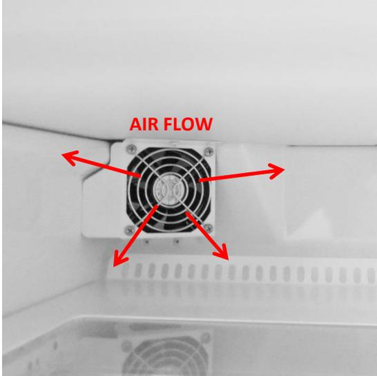
The refrigerator fan is located underneath the freezer compartment in the left rear corner.
