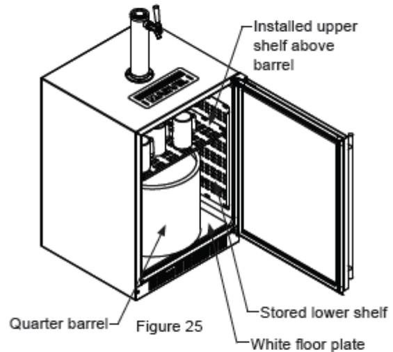
If you are using a half barrel (keg) or (2) 1/6 barrels, place the two shelves on the right side of the keg dispenser on the two mounting hooks for storage. (See Figure 26). Be sure the white floor plate is in the bottom of the interior compartment before positioning the barrel(s).
