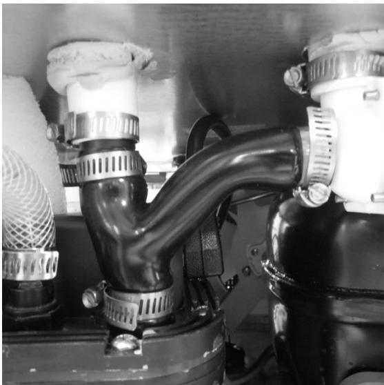
To remove the “Y” connector, disconnect:
