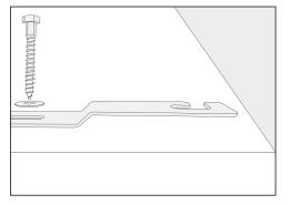
■ Install the holding bracket with the hex screws and the washers.
