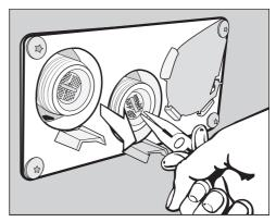
Use pointed pliers to grip the bar and pull out the filter; then clean the filter.
