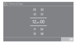
Enter the numbers by swiping upward or downward. Place your finger on the number that you want to change and move your finger in the direction you want. Use the *OK* sensor control to accept the set numerical value.
