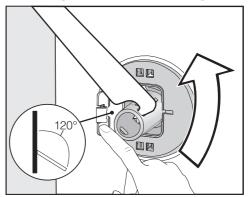
Open out the cover and use the wrench supplied with the washing machine to turn the shipping strut 90°.
