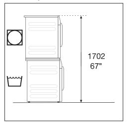
The washing machine can be installed as a washer-dryer stack together with a Miele Tumble Dryer. This requires a washer-dryer stacking kit which can be purchased separately.
