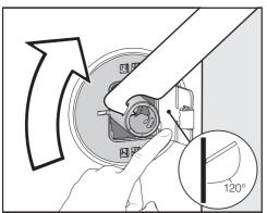
■ Open out the cover and use the wrench supplied with the washing machine to turn the shipping strut 90°.
