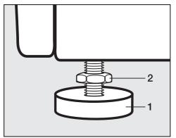
Using the wrench supplied, turn counter nut 2 in a clockwise direction.
