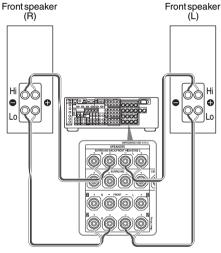
Connect the jacks on the Lo (or Hi) side of the front speakers to the FRONT A terminals, and connect the jacks on the Hi (or Lo) side of the front speakers to the SURROUND BACK/FRONT HIGH/ZONE 2 terminals. Make sure that metal fittings of Hi/Lo attached to the speakers have been removed from the speakers. Not doing so may cause a malfunction of the receiver.
