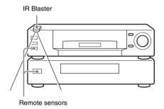
If the infrared receivers on the two components do not line up as shown in the illustration on the left, you must purchase an optional IR Blaster (VM-50, not supplied) and install it.
