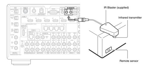
Place the components and the IR Blaster as follows when you want to operate two components with the IR Blaster.
