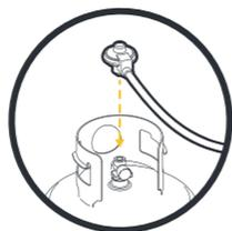
**UK:** When attaching your push fit regulator, check that the switch is in the horizontal position. Push in the button and firmly push down on to the gas valve to attach. Lift the switch to its vertical position to allow gas to flow.
