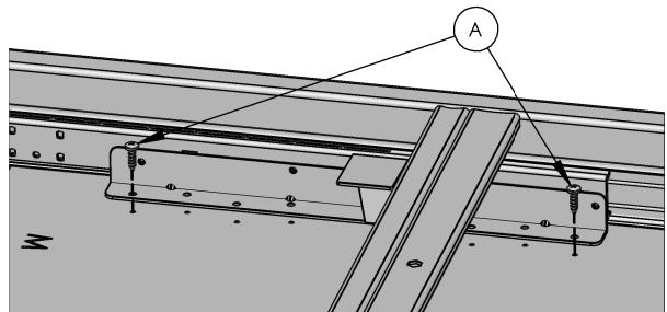
3.4 Screw firmly screws. (do not overtight)
