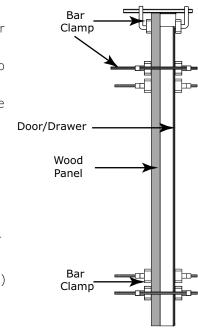
10. Using a 7/64" (3 mm) drill bit, drill 6 pilot holes into the wood panel 1/2" (12 mm)
