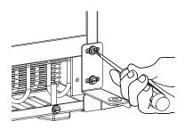
2. Remove corresponding screws on opposite side of cabinet. On some models there may be a nut behind one or both screws on either side.
