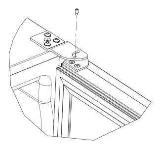
3. On 24" models, a second pin is included for the bottom hinge. Repeat steps above for second hinge.
