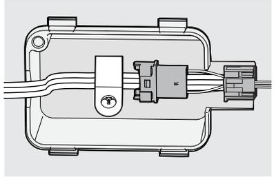
4. Reattach the electrical harness by positioning the cable clips over the black markings on the harness and push the 4 cable clips through the openings in the rail to secure the harness in place.
