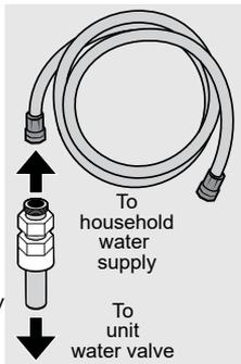
3. Open the locking clips and grab the water line coming from the refrigerator. Remove the plastic cap from the water inlet fitting and discard the cap.
