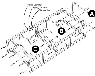
Attach Top (A), Shelves (B) and (C) with Head Cap Bolts, Spring Washers and Flat Washers.
