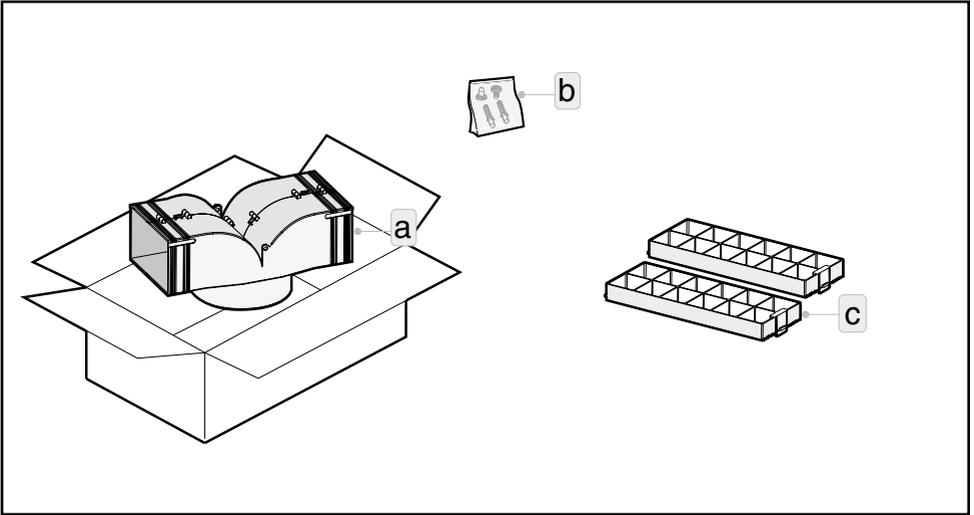
**CARBON FILTER KIT XORFK01:** The kit includes an air diverter **A**, 2 screws and 2 expansions plugs **B** and 2 rectangular filters **C**.
