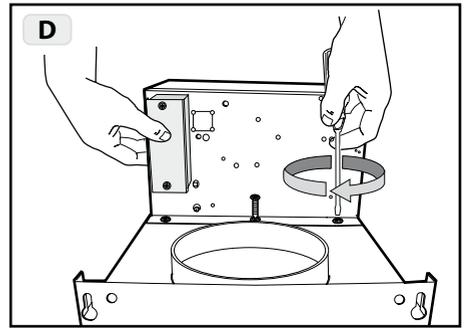
**Fig.3D:** Position the electrical box so it is in line with the holes of the previously removed screws and tighten.
