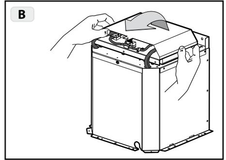
**Fig.3B:** Lift the electrical plant box.
