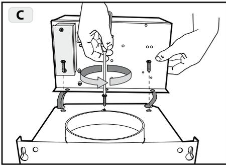
**Fig.3C:** Remove the 3 fixed screws.
