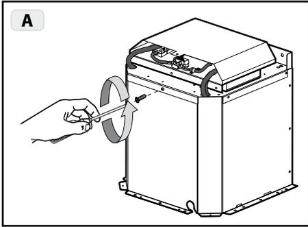
**Fig.3A:** Remove the central screw.
