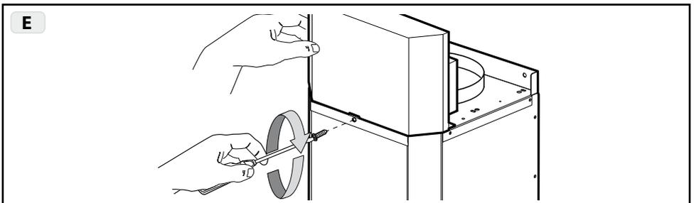
**Fig.3E:** Pay attention that the tear tape of the electrical box is inside the slot and then tighten screw.
