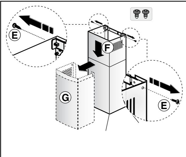
**Fig.1:** Remove the 2 screws **E** and have the top flue **F** go into the bottom flue **G**. Remove the two flues **F-G** and place them on a flat surface.
