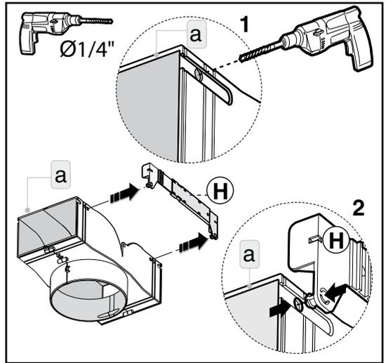
**Fig.4:** Take the air diverter **A** and drill two holes as shown in the figure (hole diameter: **1/4" inches**). Once the two holes have been drilled, fasten the air diverter **A** to the bracket **H**.
