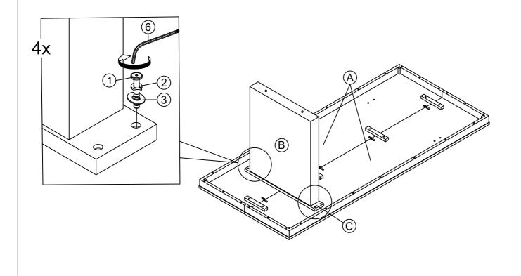
STEP 6 : Assemble the rail (D) to the the leg frames by using the Allen Key (6) and the hardware Bolt 1/4" x 2" (2), Spring washer (3) & Flat washer (4).
