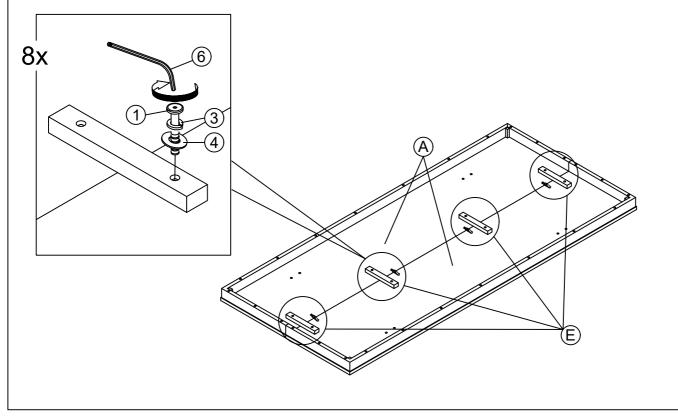
STEP 3 : Assemble the mounting plate (C) to the table leg (B) by using the Allen Key (6) and the hardware Bolt 1/4" x 1 3/16" (1), Spring washer (3) & Flat washer (4).
