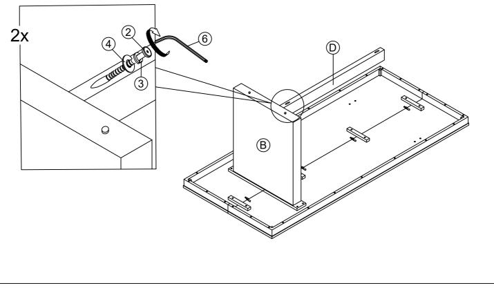
STEP 7 : Assemble the leg frames to the table top (A) & rail (D) by using the Allen Key (6) and the hardware Bolt 1/4" x 1 3/16" (1), Bolt 1/4" x 2" (2), Spring washer (3) & Flat washer (4).
