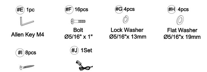
Screw #4 x 30mm Plug-in-Power Supply
