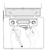
3. Remove the Wall bracket install guide.
