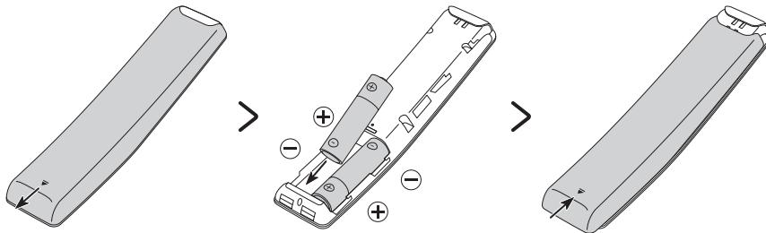
To install the batteries, push the rear cover open in the direction of the arrow at the bottom of the illustration, and then insert the batteries as shown in the figure. Make sure that the positive and negative ends are facing in the correct direction. Close the rear cover as shown.
