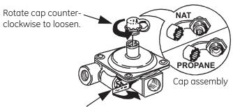
Lever shown closed (Oven Shut Off only) FLIP LEVER UP TO OPEN
