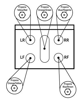
To prevent leakage, make sure the orifices are securely screwed into the gas supply tubes.
