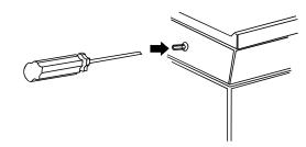
Center adjustment screw for all burners.
