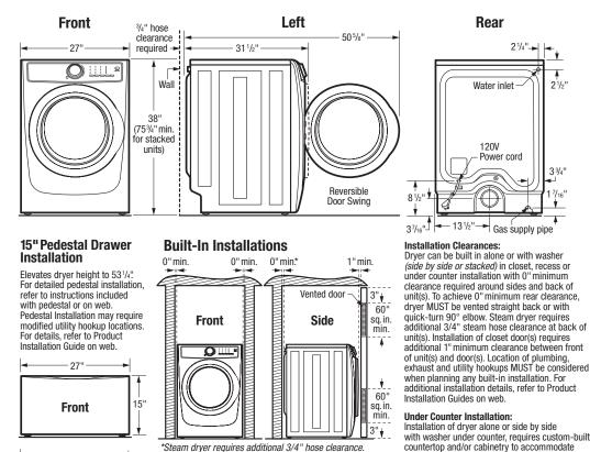
with washer under counter, requires custom-built countertop and/or cabinetry to accommodate unit(s) height
