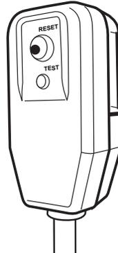
Power cord includes a current interrupter device. A test and reset button is provided on the plug case. The device should be tested on a periodic basis by first pressing the TEST button and then the RESET button while plugged into the outlet. If the TEST button does not trip or if the RESET button will not stay engaged, discontinue use of the air conditioner and contact a qualified service technician.
