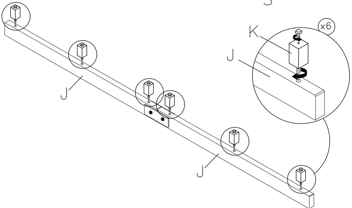
Turn Adjustable Leveler on the bottom of the Cross-Slat Support Leg leaving 6mm space between leveler and the floor.
