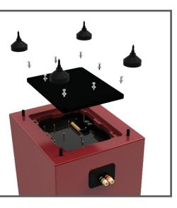
same process as above, lengthen the appropriate spikes on the left or right of the SabrinaX until it is level.
