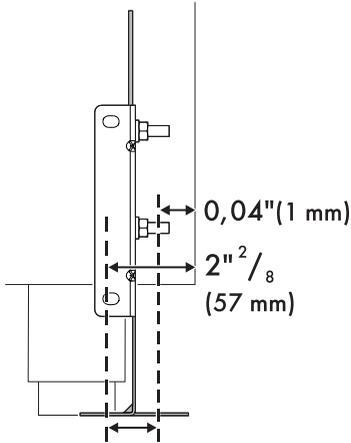
8. After having positioned and leveled the appliance, move the bracket close to the rear of the appliance and anchor it to the floor using the two washers and screws. A qualified technician must verify the suitability of the materials in accordance with the type and condition of the floor.
