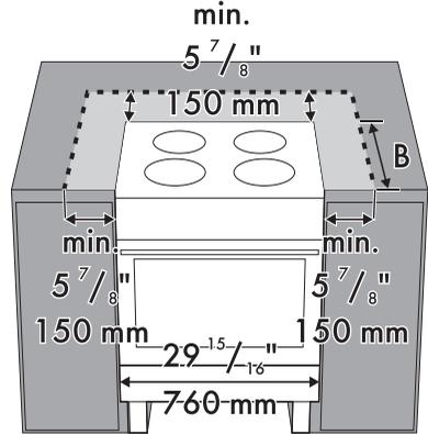
The side cabinet depth (clearance **B**) must match the front edge of the range side panel.
