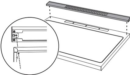
2. Secure the backguard to the top by tightening screws.
