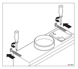
Loosen the retaining bracket screws and push the brackets back against the rear wall.
