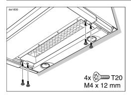
■ Secure the hood to the brackets from below using two screws on each side.
