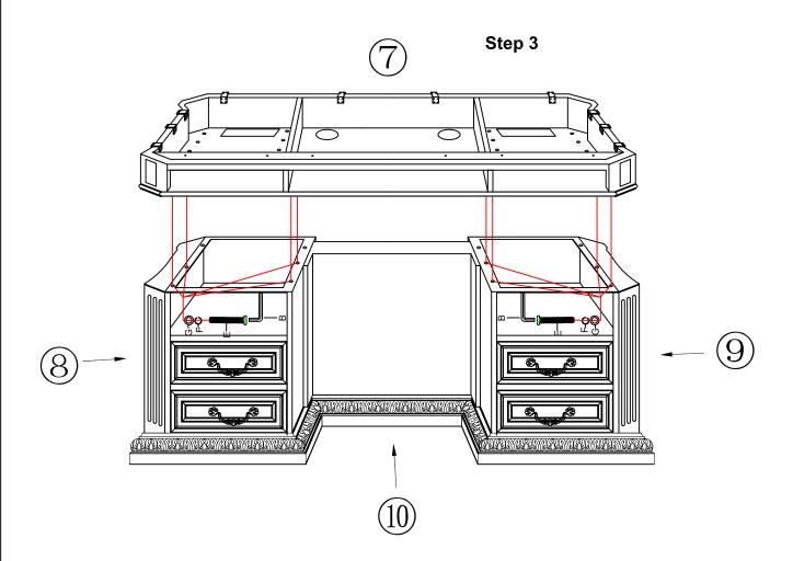
Step 3: Loosen the remaining 4 bolts (E), lock washers (F), flat washers (G) attached at wood cleats under left bottom panel by using allen wrench (B) from the bottom, and then repeat the steps at right base (9), then take off the top section(7).
