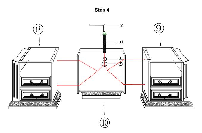
Step 4: loosen four bolts (E), lock washers (F), flat washers (G) attached the back panel (10) to the desk with allen wrench (B) and separate back panel (10) by pulling it upright.
