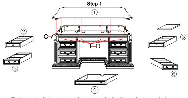
Step 1: Take out all three top drawers (2, 3, 4) and second drawers (5, 6) on both sides, loosen all screws (C) on L-shaped metal plates and screws (D) under the front edge of top panel (1), and remove top panel (1) from desk.
