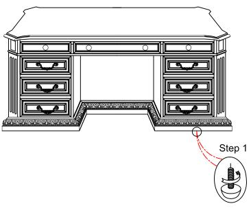
Adjust Leveler if needed to level desk on uneven floor.
