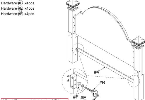
Align HB support (#4) to the HB legs, then secure by using bolts (#B) with washers (#E,F).
