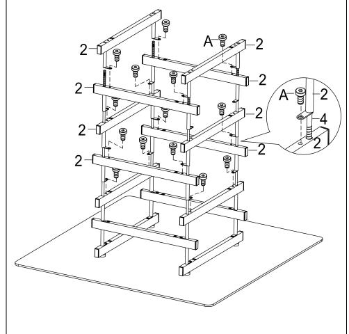
\*Repeat **STEP 3**; insert all stretchers (2) to build up the frame as shown.
