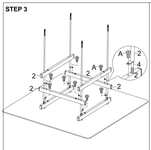
Insert attached long bolts (4) through the corresponding holes on stretchers (2) as shown and fix stretchers (2) to stretchers (1) by using bolts (A) as shown.
