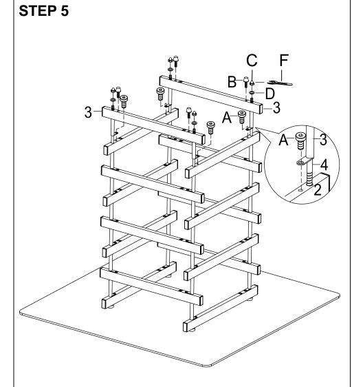
Attach stretchers (3) to stretchers (2) by using bolt (A) as shown then tighten all bolts firmly.
