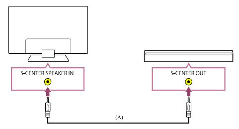
(A) TV center speaker mode cable (supplied with sound bars that have S-CENTER OUT terminals)
