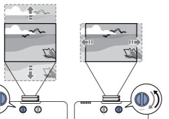
2. If the projector is on a table, you can level the image by turning any of the projector's adjustable feet.
