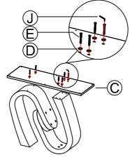
Step 3 Attach the bottom plate to the pedestal
