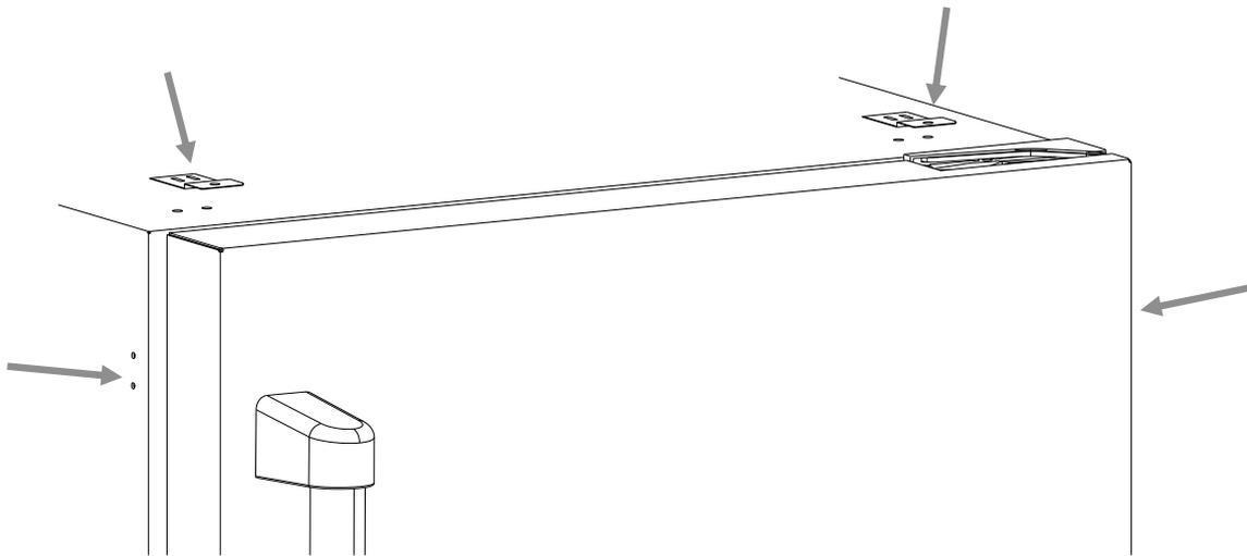
1. Once you've determined the appropriate height and have ensured the appliance is level, position the unit at the front of the cutout to install the anti-tip system, which is necessary to reduce risk of tipping.
