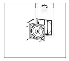
Figure 8.2: Inserting the Baffle
