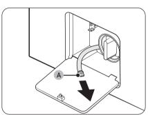
3. Put an empty, spacious container around the cover, and stretch the emergency drain tube to the container while holding the tube cap (A).
