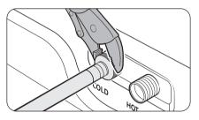
4. Attach the water hoses to the hot and cold water inlets on the back of the washer, and then hand tighten the water hose fittings until they are tight. Then, use pliers to tighten the fittings by an additional two-thirds of a turn.
