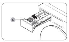
4. Turn the Dispenser 2 cap (C) anticlockwise to open.
