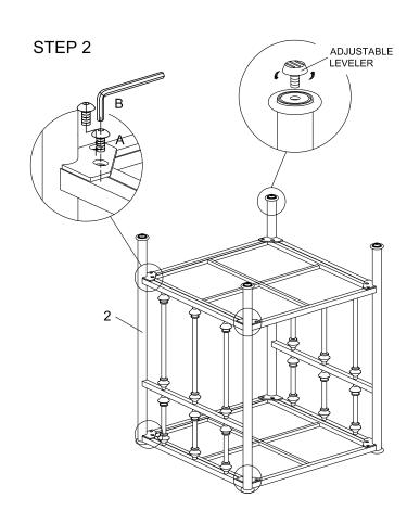
NOTE: DO NOT TIGHTEN ALL THE BOLTS UNTIL THEY ARE INSTALLED IN CORRESPONDING HOLES!
