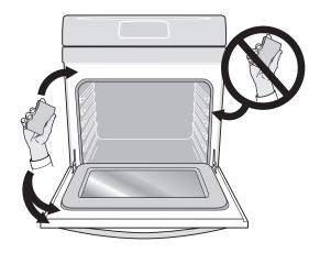
Figure 23: Clean around the oven door gasket Notes:
