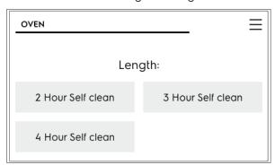
Do not open the oven door while the lock motor is running or when any locking indicators or displays are showing. The oven door is completely locked in about 4 seconds. Once the oven door has locked, CLEAN will appear in the display indicating self clean has started.
