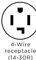
Use a 4-wire power supply cord with ring terminals and UL listed strain relief. The 4-wire power supply cord, at least 4.92 ft. (1.5 m) long, must have 4 10-gauge solid copper wires and match a 4-wire receptacle of NEMA Type 14-30 R, rated 120/240V, min 30A. The ground wire (ground conductor) may be either green or bare. The neutral conductor must be identified by a white color.
