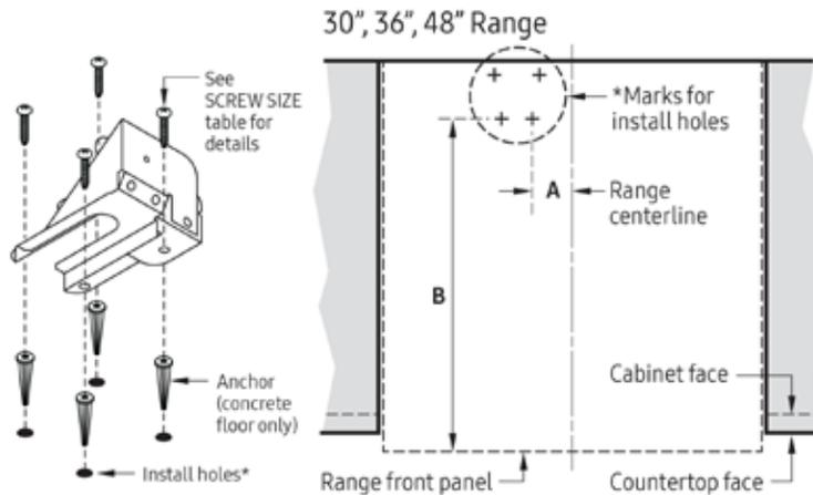
1. Drill four  $\frac{3}{8}$ " dia. countersink holes through the flooring but not into the concrete.
