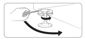
**3.** When levelling is complete, tighten the nuts using the wrench.
