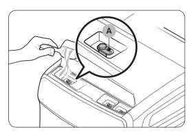
2. Add a recommended amount of liquid or powdered detergent to the detergent compartment. Do not exceed the max line (A).
