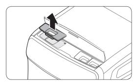
1. Open the top-front cover. Grasp the main wash compartment, and then pull up to remove.
