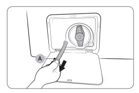
**3.** Put an empty, spacious container in front of the cover, and stretch the emergency drain tube to the container while holding the tube cap (A).
