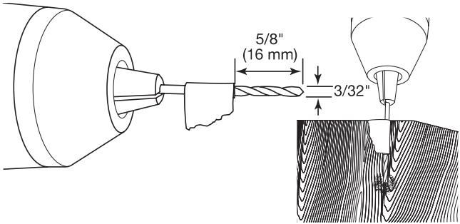
**NOTE:** Do not drill deeper than 5/8" (16 mm) to keep from drilling through panel. Pilot hole depths given are for 3/4" (19 mm) thick panel.
