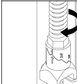
Each hinge has 3 different spring tension levels that it can be set to. The current tension level is indicated by an arrow. 1 is the lowest spring tension for light doors and 3 is the highest for heavier doors. 2 is the middle tension for door panel weights that fall between heavy and light.
