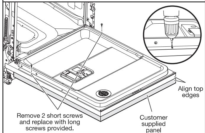
Remove the short screws (4<sup>th</sup> from top) on either side of the inner door panel. Use tape to mark a 3/32" drill bit to gauge the hole depth of approximately 1 1/2" (38 mm). Drill 2 pilot holes using the door liner hole as a guide into the panel. Install the 2 remaining long screws.
