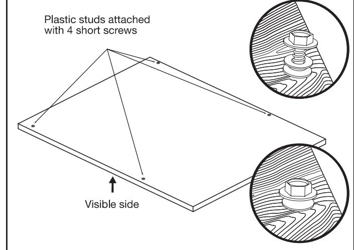
Attach the 4 plastic studs to the wooden panel using the four 5/16" hex-head (short) screws provided.
