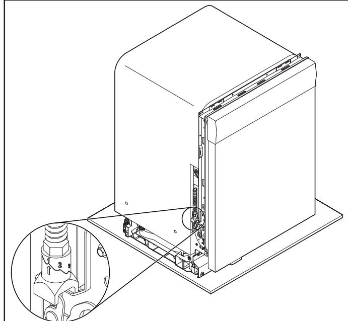
With the dishwasher partially or fully removed from the cabinet, the hinge spring tension adjusters can be accessed at the front sides of the dishwasher.
