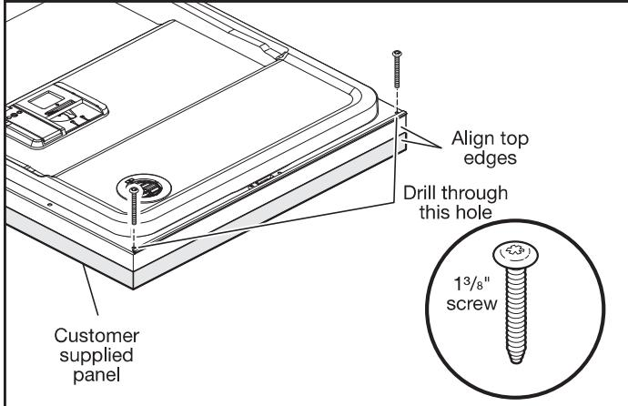
Using a Torx T15 screwdriver, install two #8 x 1 3/8" (long) screws in top corners to secure custom wood panel in place.
