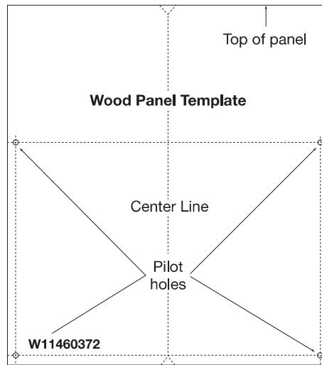
Using the template provided, attach it to the backside of the custom panel with tape. Make sure that the center of the template is aligned with the center of the wooden panel and top of the template is aligned to the top face of the wooden panel.
