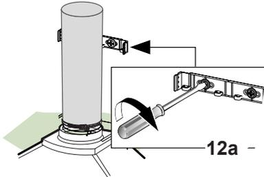
Only for the recirculation version, connect the hood to the Air outlet.
