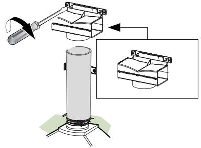
Fix the Ductless Diverter with two screws 12a supplied as shown.
