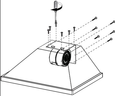
Once the blower is in place re-install the 12 screws to fasten the motor to the Hood body.
