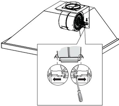
Disconnect the Electrical Connectors by depressing the tabs with your hand and also using light force on one tab with a flat head screwdriver.
