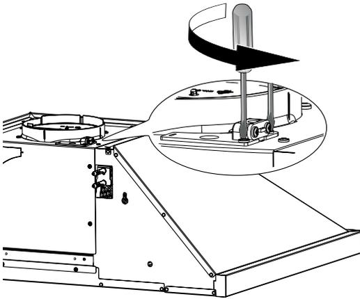
Remove the 2 screws as shown in the image to the left from the top electrical cover and set aside.
