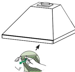
Replace the metal grease filters removed previously.
