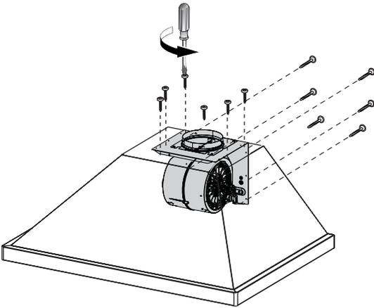
For a horizontal ducting installation the motor needs to be unsecured by first removing the 12 screws as shown.
