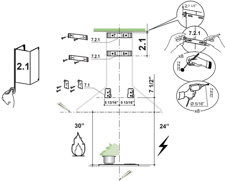
Place a Upper bracket 7.2.1 on the wall as shown about  $1 \frac{1}{8}$ " from the ceiling or upper limit, aligning the centers(notch) with the vertical reference line and mark the wall at the centers of the holes in the bracket. Place the other bracket 7.2.1 on the wall as shown, below the first bracket, at the height of the upper chimney section supplied and aligning the centers(notch) with the vertical line.
