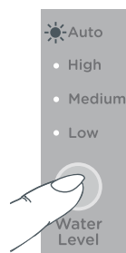
Fig.24 Selecting AUTO water level
