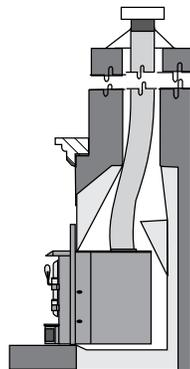
1. When installed in a factory built fireplace, a full stainless steel rigid or flexible flue liner is mandatory, for both safety and performance purposes. When a flue or liner is in use, the insert is able to breathe better by allowing a greater draft to be created. The greater draft can decrease problems such as, difficult start-ups, smoking out the door, and dirty glass.
