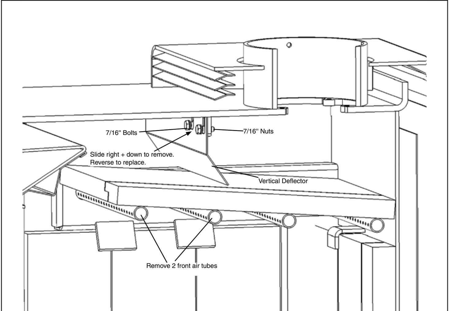
1. Remove 2 front secondary air tubes / vermiculite baffles as per page 15.
