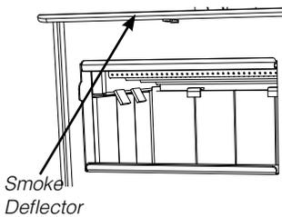
2. Slide the left baffle over the 2 remaining air tubes from the front and then push it to the back.
