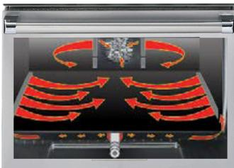
Balanced heat distribution is essential when baking, roasting, and dehydrating food. The American Range convection oven technology features a convection motor and louvered side panels to enhance uniform heat distribution throughout the large oven cavity. The strategic placement of the convection fan ensures consistent heat distribution.
