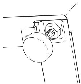
**NOTE:** To minimize vibration, the locking nuts must be tight.
