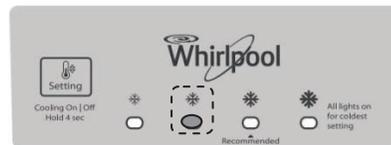
The median minimum temperature will be displayed when you press the Setting button once from the least-cold temperature. The second indicator will be ON.
