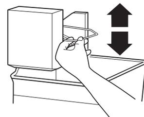
**NOTE:** Turn the ice maker off before removing the ice storage bin to serve ice or to clean the bin. This will keep the ice cubes from dropping out of the ice maker and into the freezer compartment. After replacing the ice storage bin, turn on the ice maker.
