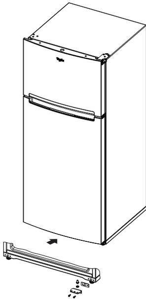
2. Open both doors again to make sure they close as easily as you like. If not, tilt the refrigerator slightly more to the rear by turning both leveling legs to the left; it may take several more turns.
