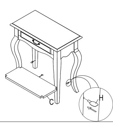
Step 3 Now tighten the bolts in Step 1 and put the drawer back into the table.
