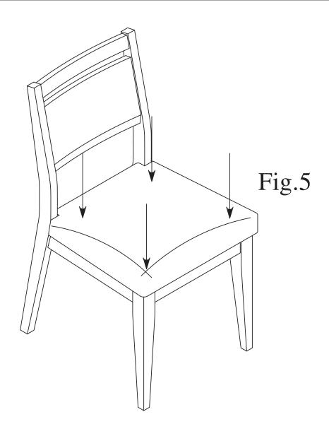
Step 3: Place the loosely assembled chair to an upright position on a hard flat surface and apply gentle downward pressure on the seat. As shown on Fig.5. Once the chair is balanced and leveled, fully tighten all bolts.
