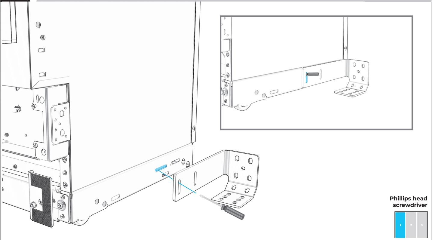
**3.4** LOOSELY ATTACH POSITIONING BRACKET TO MOUNT.
