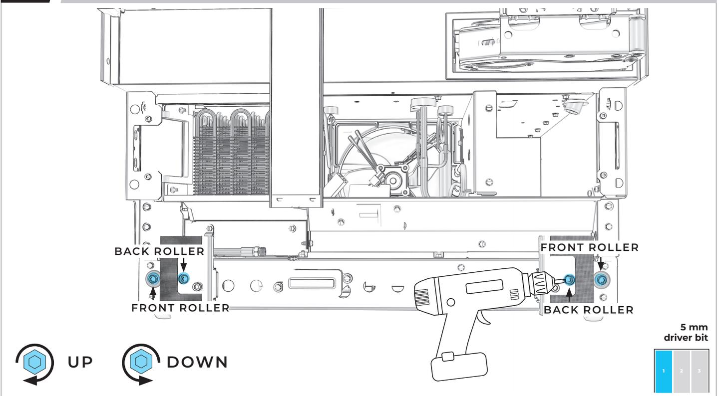
6.9 LOOSELY DRIVE SCREWS THROUGH INSTALLATION BRACKET AND BADASS SOFFIT BRACKET.
