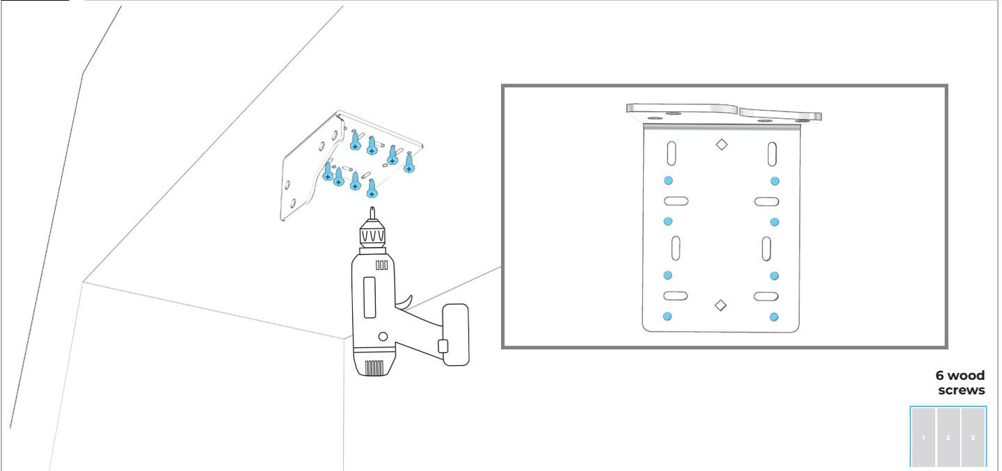
★ A MINIMUM OF SIX SCREWS MUST BE USED TO SECURE BRACKETS TO CABINET. FAILING TO PROPERLY SECURE BRACKETS CAN RESULT IN A TIP HAZARD.
