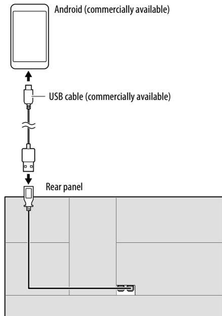
When connecting an Android device, "HAND MODE" is shown. You can control Android device using a media player application installed in the Android device.
