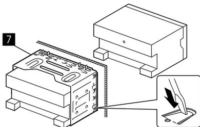
Bend the tabs of the mounting sleeve with a screwdriver or similar utensil and attach it in place.
