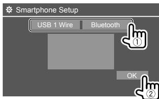
**[USB 1 Wire]** Select this when the device is connected via the USB input terminal (cable from the rear panel).
