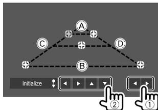
Make sure that **A** and **B** are horizontally parallel, and that **C** and **D** are the same length.
