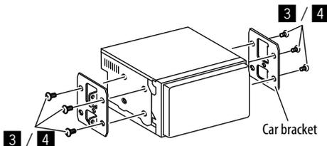
**Note:** Select the appropriate screws (supplied) for the mounting bracket.
