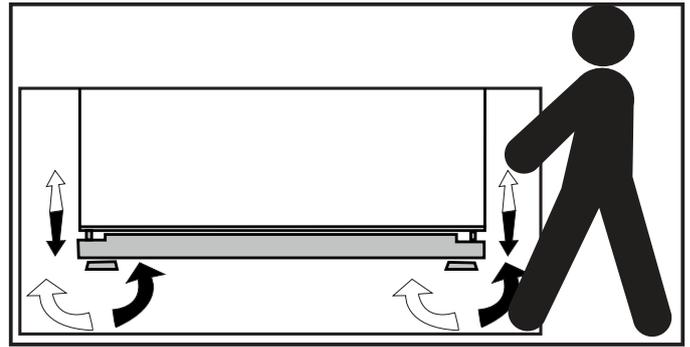
Turn the front feet to balance the product. The corner where the foot exists is lowered when you turn in the direction of arrow and raised when you turn it in the opposite direction.
