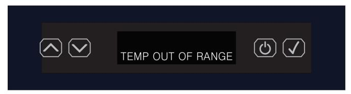
The TEMP OUT OF RANGE alert activates when the temperature level is out of range by 10 degrees Fahrenheit for a 12-hour time period.
