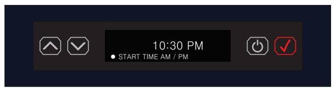
18. Once the start time is properly set, set the END TIME HOUR for the SCHEDULE NIGHTLIGHT by pressing the UP or DOWN ARROW buttons.
