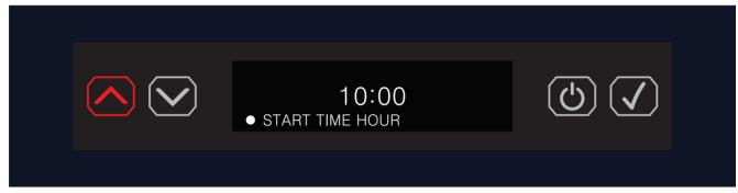
13. Once the hour is set, press the ENTER button ( $\checkmark$ ).
