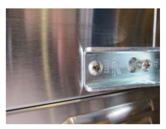
4. Remove the inner top and bottom right-side hinge screws. Install these screws about three turns in the left-side outer top and bottom screw locations.
