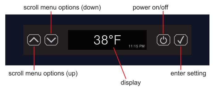
NOTE: The clock time only displays if the user has set the NIGHTLIGHT function; otherwise the clock time does not appear on the screen.
