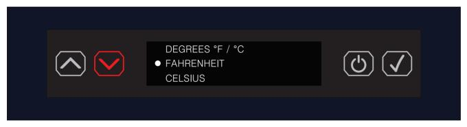
4. The default unit setting is DEGREES FAHRENHEIT (°F). To maintain the DEGREES FAHRENHEIT (°F) setting, press the ENTER button ( ✓ ).
