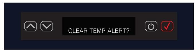
3. The display reverts back to the default display and the TEMP OUT OF RANGE alert clears.
