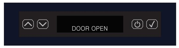
NOTE: The audible alert emits three beeping sounds that occur every 30 seconds after the door has remained open for more than 2 minutes. The alert automatically clears when you properly close the door. This methodology applies to any error or alert that requires an audible alert.
