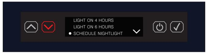
3. Set the clock time before reaching the desired SCHEDULE NIGHTLIGHT setting. Press the ENTER button ( $\checkmark$ ).
