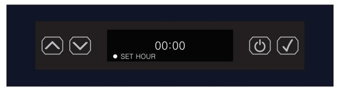
5. Set the hour using the UP / DOWN ARROW buttons.
