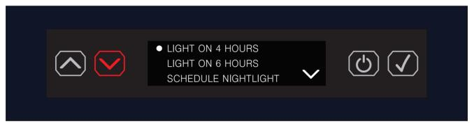
4. To return back to the main menu, scroll down by pressing the DOWN ARROW ( ) and then press the ENTER button ( ).
