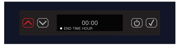
19. Using the UP / DOWN ARROW buttons, select the END TIME HOUR.
