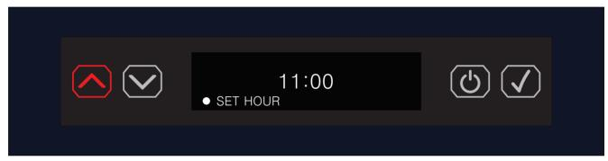
6. Once the hour is set, press the ENTER button ( $\checkmark$ ).
