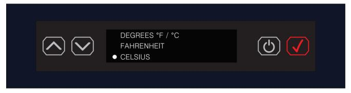
NOTE: DEGREES FAHRENHEIT (°F) is the default setting and displays in increments of 1 degree. DEGREES CELSIUS (°C) displays in increments of 0.5 degrees.
