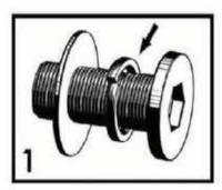
When lock or spring washer is used in an assembly, please make sure the lock or spring washer is placed between the larger flat washer and the head of the screw or bolt.
