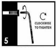
Make sure all parts are properly aligned, then use the appropriate hand tool to completely tighten the bolts or screws. Do not use power tools and do not overtighten.
