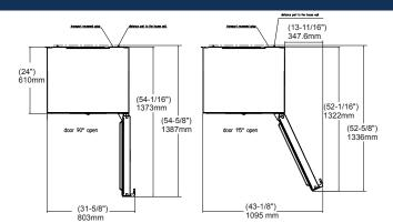
Allow door swing clearance at locations next to a wall. If the appliance is installed with the hinges next to a wall (4), the distance between the appliance and the wall must be at least  $1\frac{1}{2}$ " (40 mm). This is how far the handle protrudes when the door is open.
